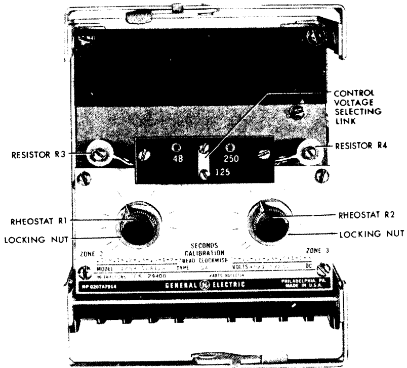
Figure 1A (8039885) Relay Type SAM16A12A Removed from Case (Front View)
