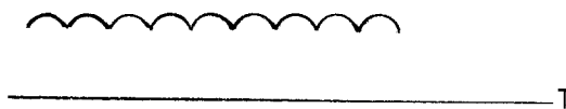
FIG. 10 (0246A2274-0) CURRENT DETECTOR LEVEL DETECTOR INPUTS PRODUCED BY SINGLE PHASE AND THREE PHASE CURRENTS FOR THE SBC41A RELAY
