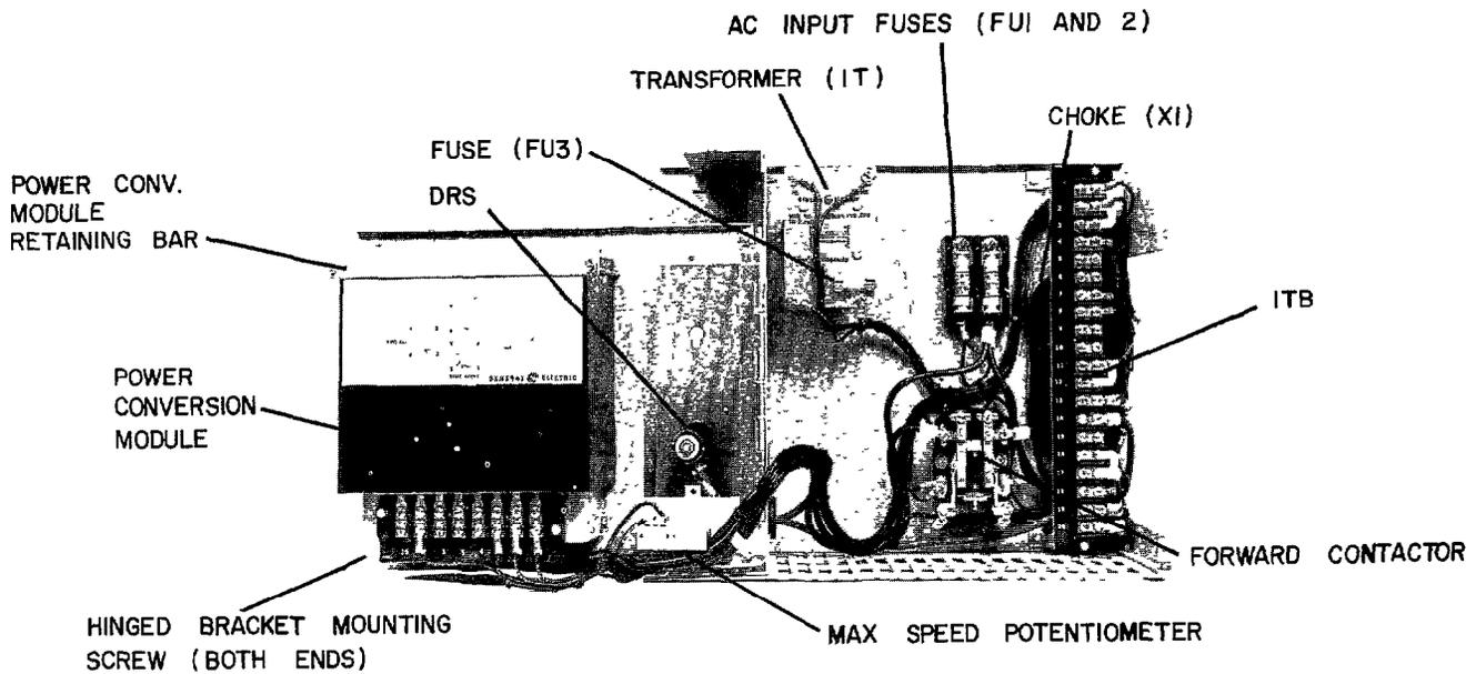
POWER UNIT ASSEMBLY – BASIC, NON-REVERSING, HINGED PANEL OPEN
