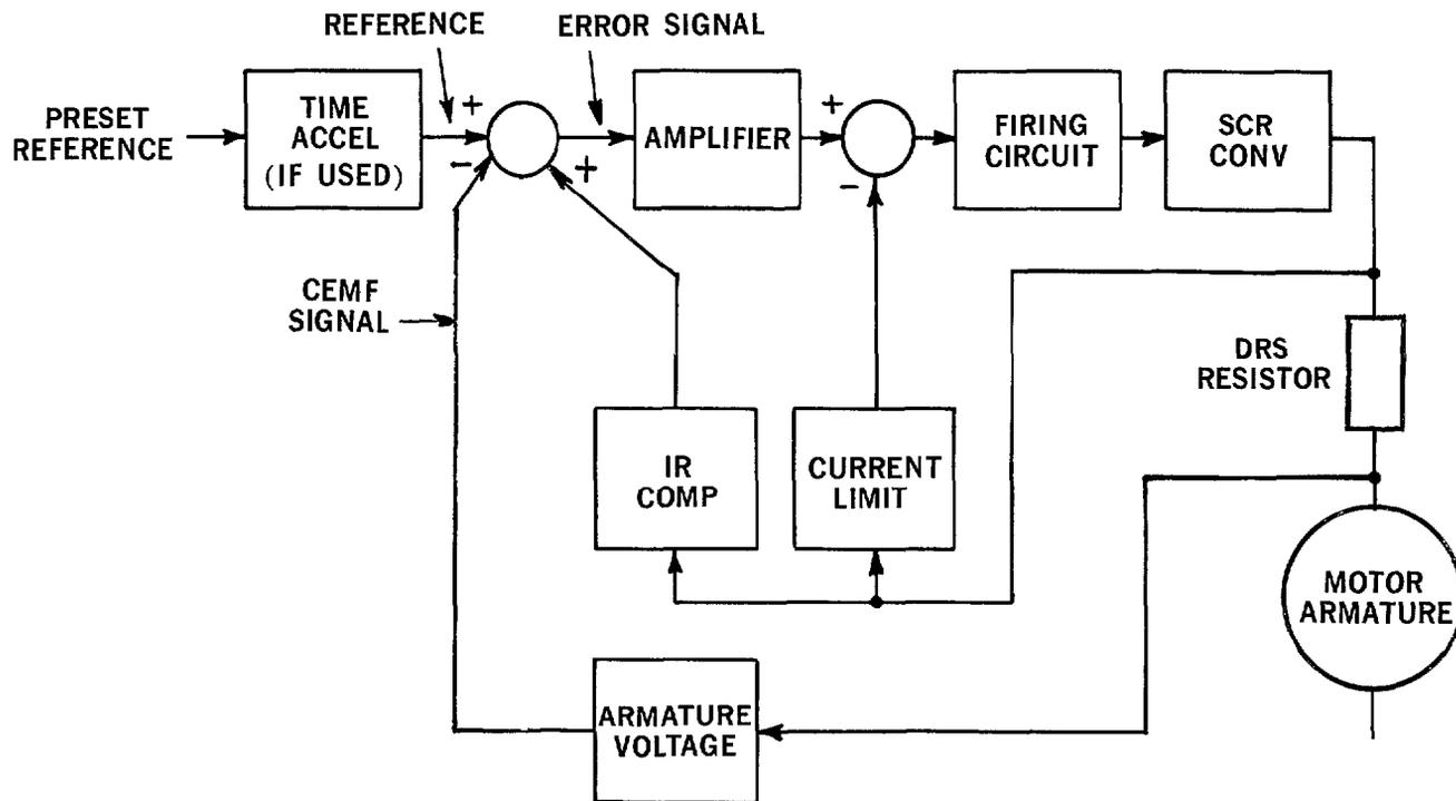
Figure 7 Regulator Block Diagram
