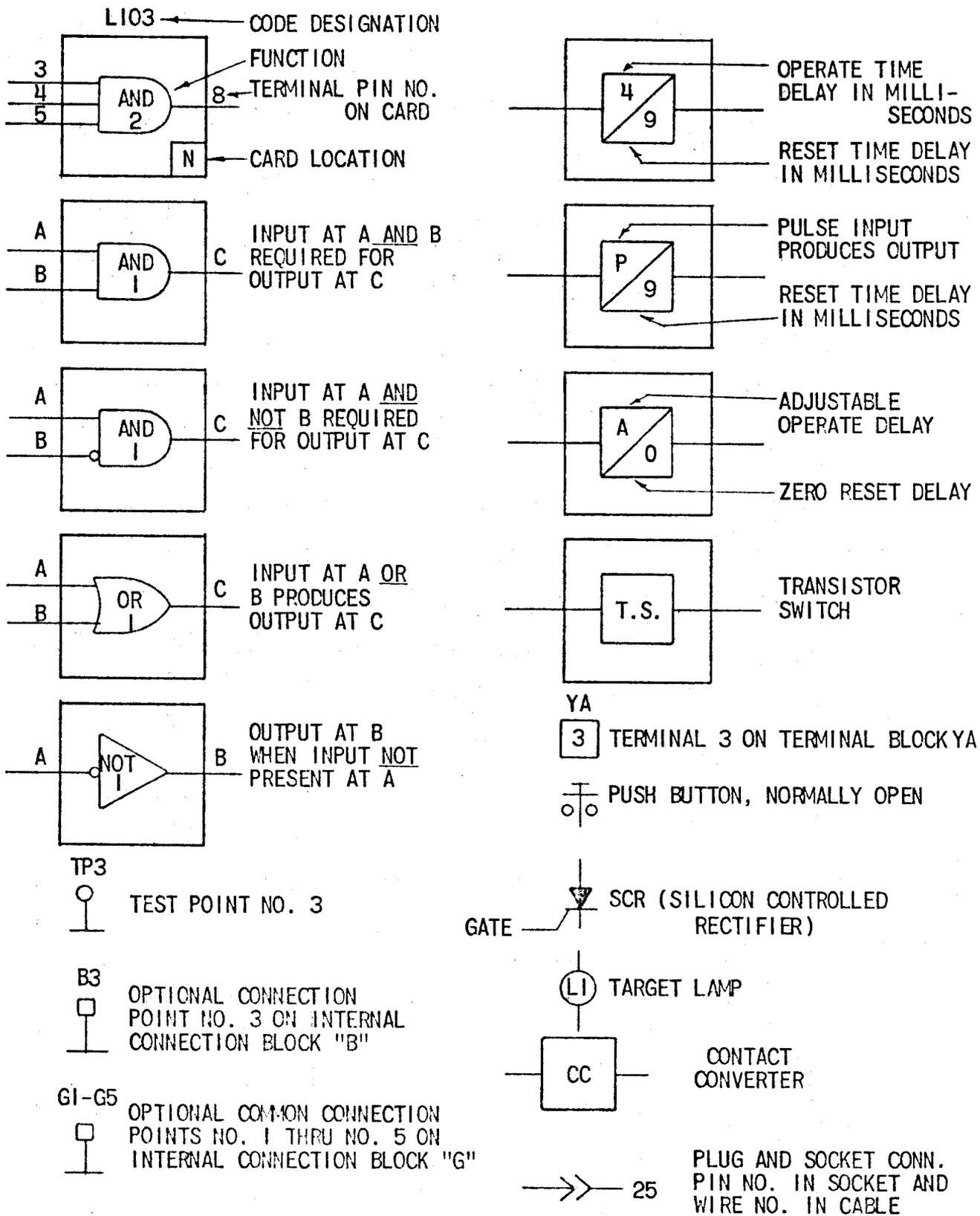
FIG. 4 (0227A2047-0) Logic And Internal Connection Diagram Legend
