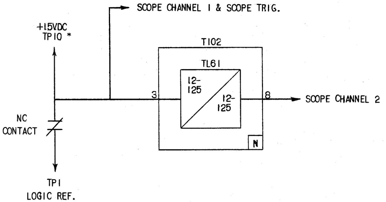
\* THE 15VDC SIGNAL AT PIN 10 HAS A CURRENT LIMITING RESISTOR MOUNTED ON THE TEST CARD.
