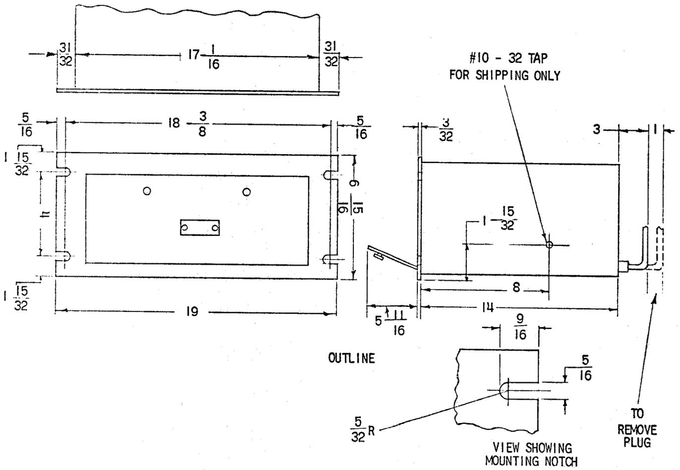
FIG. 1 (0227A2037-0) Outline And Mounting Dimensions For The Type SLA52A Relay
