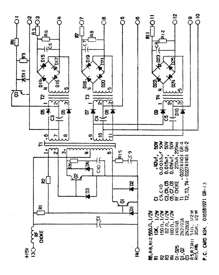
FIG. 4 (0208A5504AJ-1 ) ISOLATION INTERFACE FOR CS26B
