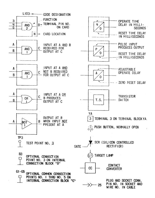
FIG. 2 (227A2O47-0 ) LOGIC AND INTERNAL DIAGRAM LEGEND
