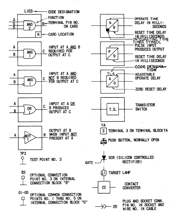
FIG. 4 (227A2047-1 ) LOGIC AND INTERNAL CONNECTION DIAGRAM LEGEND
