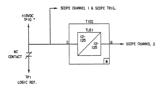
\* THE 15VDC SIGNAL AT RIN 10 HAS A CURRENT LIMITING RESISTOR MOUNTED ON THE TEST CARD.
