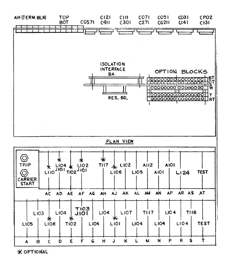
FIG. 2 (257A8713-1 ) COMPONENT LOCATION DIAGRAM FOR THE SLA51G RELAY
