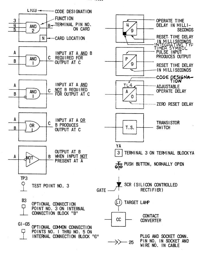
Fig. 2 (0227A2047-1) Internal Connection Diagram Legend
