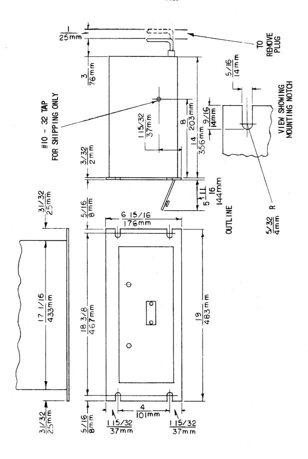
Fig. 4 (0227A2037-1) Outline and Mounting Dimensions for the Type SLA52H Relay
