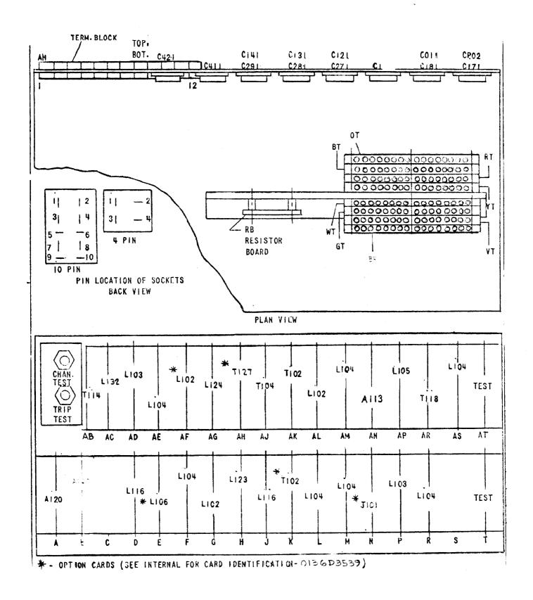
Fig. 5 (0269A3132-0) Component and Card Locations for the SLA52H Relay
