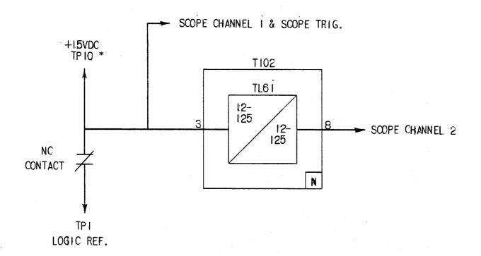
\* THE 15VDC SIGNAL AT PIN TO HAS A CURRENT LIMITING RESISTOR MOUNTED ON THE TEST CARD.
