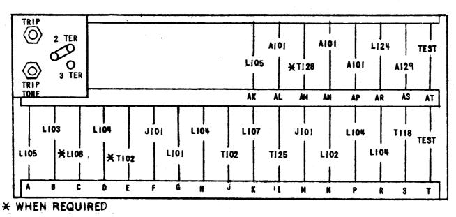
Fig. 3 (0257A6172-0) Component Locations for the Type SLA54C Relay
