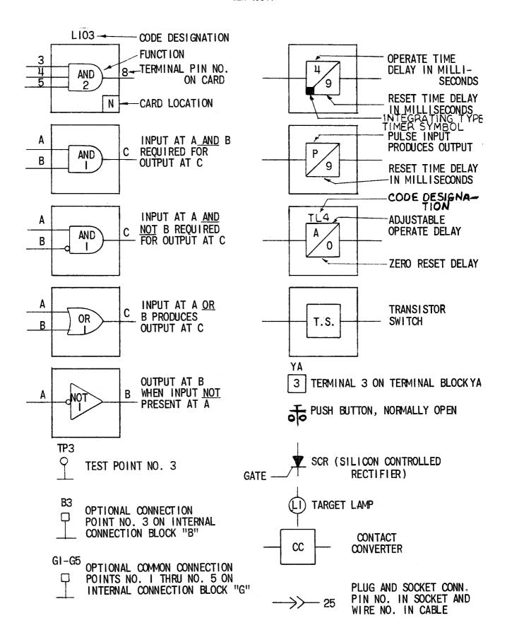
Fig. 4 (0227A2047-1) Logic and Internal Connection Diagram Legend
