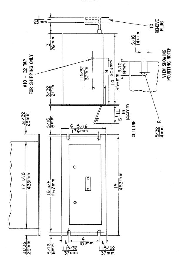
Fig. 1 (0227A2037-1) Outline and Mounting Dimensions for the Type SLA54C Relay
