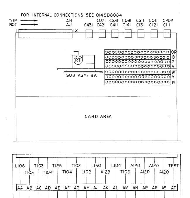
Fig. 3 (0285A5756-0) Component Location Diagram for the Type SLA54G Relay.
