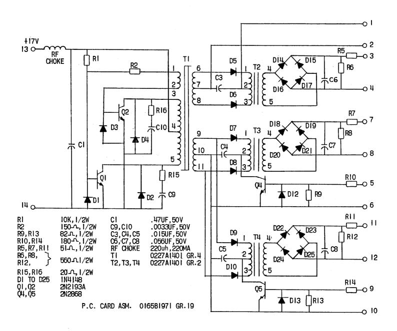
Fig. 6 (0208A5504AR-0) Internal Connections for the Isolation Interface Used in the Type SLA54G Relay
