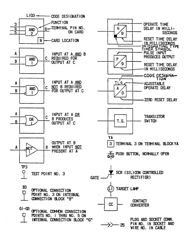
Fig. 4 (0227A2047-1) Logic and Internal Connection Diagram Legend
