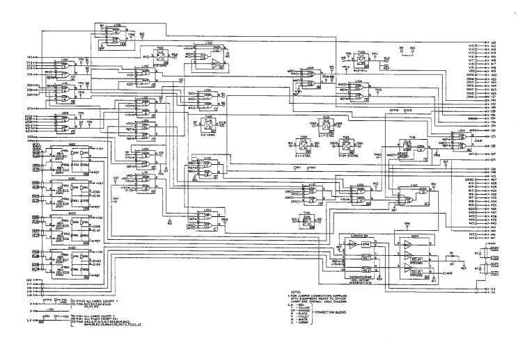
Fig. 2 (0145D8084-1) Internal Connections for the Type SLA54G Relay
