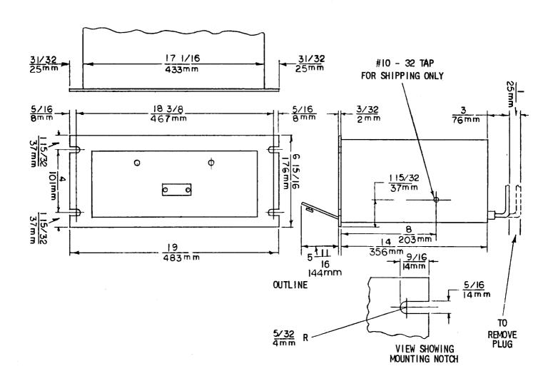
Fig. 1 (0227A2037-1) Outline and Mounting Dimensions for the SLA54G Relay
