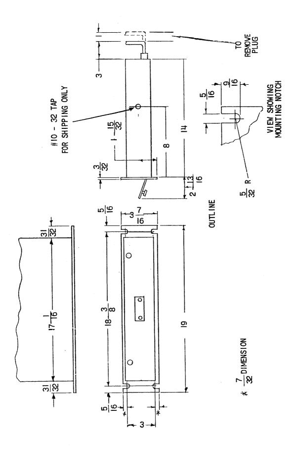
Figure 1 - (0227A2036) Outline and Mounting Dimensions for Type SLA56E Relay
