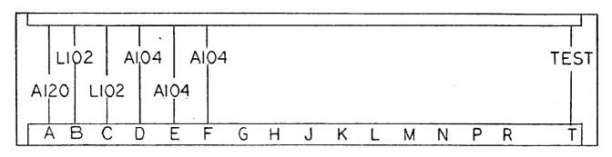
Figure 3 - (0285A9124) Component and Card Locations for the Type SLA56E Relay
