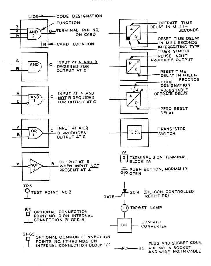
Figure 4 - (0227A2047) Internal Connections Diagram Legend
