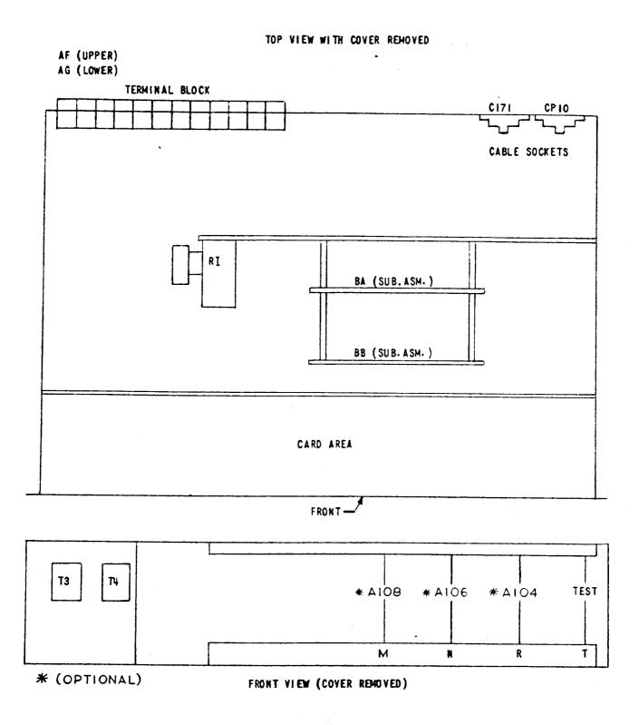
Figure 2 (0286A2022) Component Locations for the SLAT52A, Forms 20 and Up
