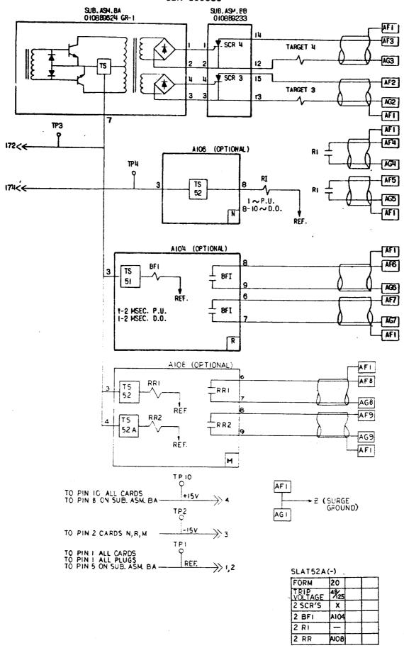
Figure 1 (0184B5796) Internal Connection Diagram for the SLAT52A Relay Forms 20 and Up
