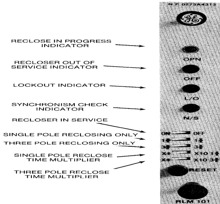
Figure 23 (8043727-0) Front View Photograph of RLM101 Module
