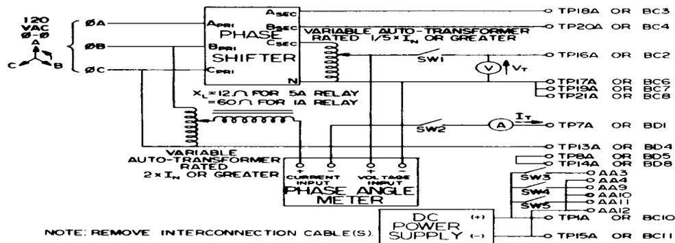
Figure 61 (0285A7576-0) Test Circuit for Auxiliary Functions Requiring Contact Inputs
