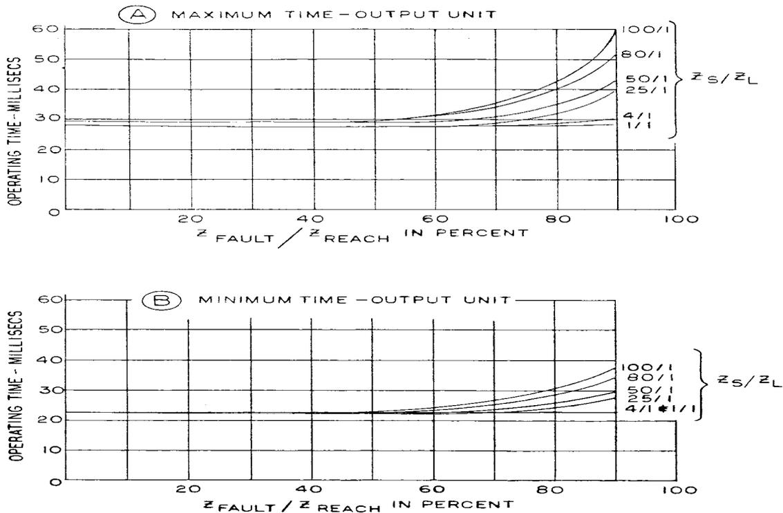
Figure 72 (0285A6680-1) Constant  $Z_S / Z_L$  Time Curves - Phase-to-Ground Faults
