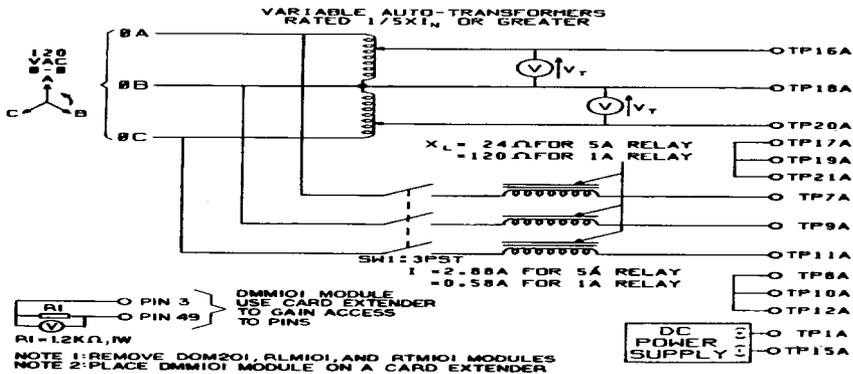
Figure 54 (0285A7582-0) Test Circuit for Post-Installation Out-of-Step Blocking Test
