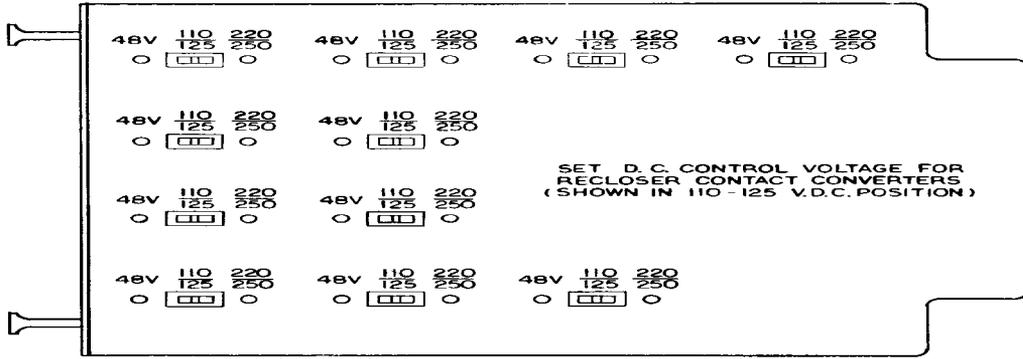
Figure 37 (0285A6625-1) Internal Links - ROM101 Module
