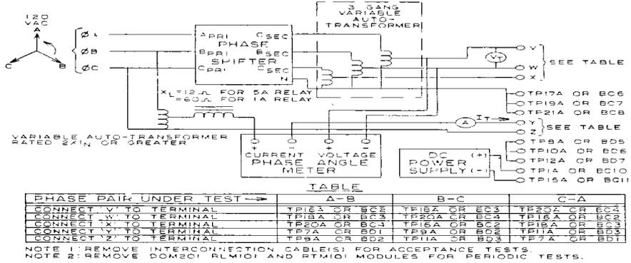
Figure 50 (0285A6610-2) Test Circuit for Phase-to-Phase Reach Tests
