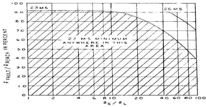
Figure 79 (0285A6685-1) Constant Time Operating Curves - Three Phase Faults (Minimum)
