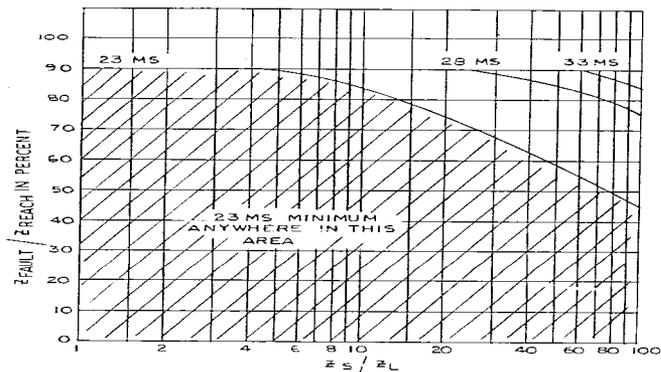
Figure 75 (0285A6682-1) Constant Time Operating Curves - Phase-to-Ground Faults (Minimum)
