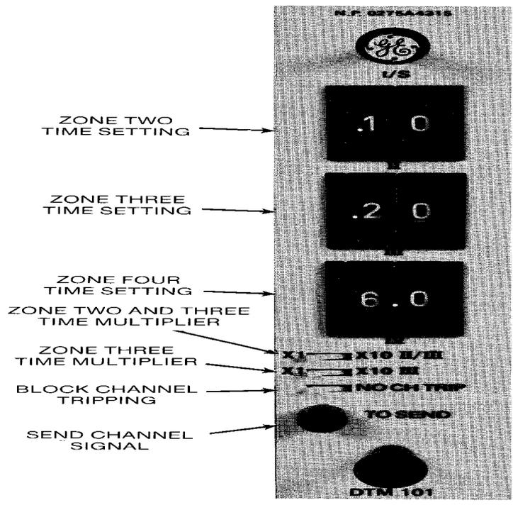
Figure 20 (8043730-0) Front View Photograph of DTM101 Module
