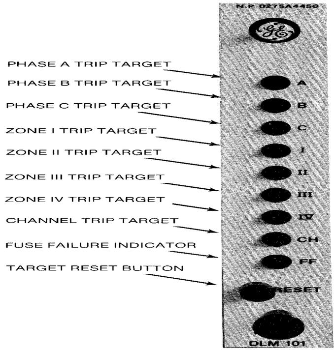
Figure 17 (8043728-0) Front View Photograph of DLM101 Module
