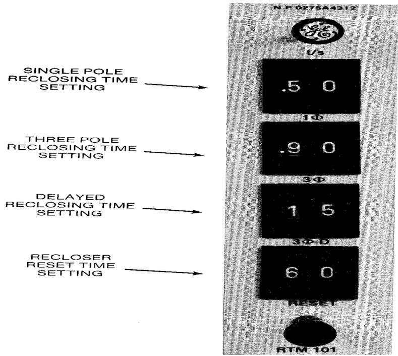
Figure 24 (8043726-0) Front View Photograph of RTM101 Module
