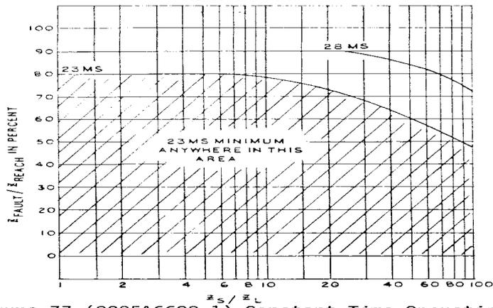
Figure 77 (0285A6688-1) Constant Time Operating Curves - Phase-to-Phase Faults (Minimum)
