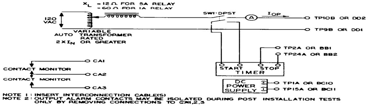
Figure 67 (0285A7578-0) Test Circuit for Non-Directional Ground Time Overcurrent Function
