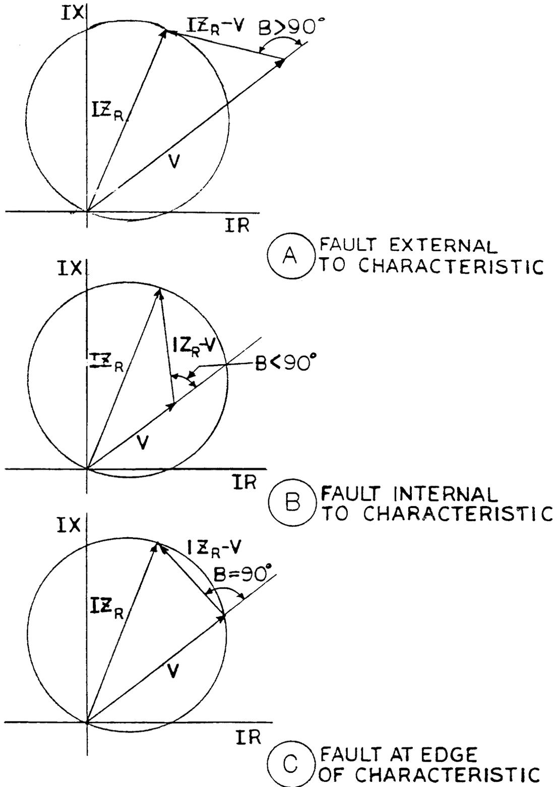
Figure 3 (0285A6690-0) Voltage Diagrams of Circular Mho-Type Characteristic
