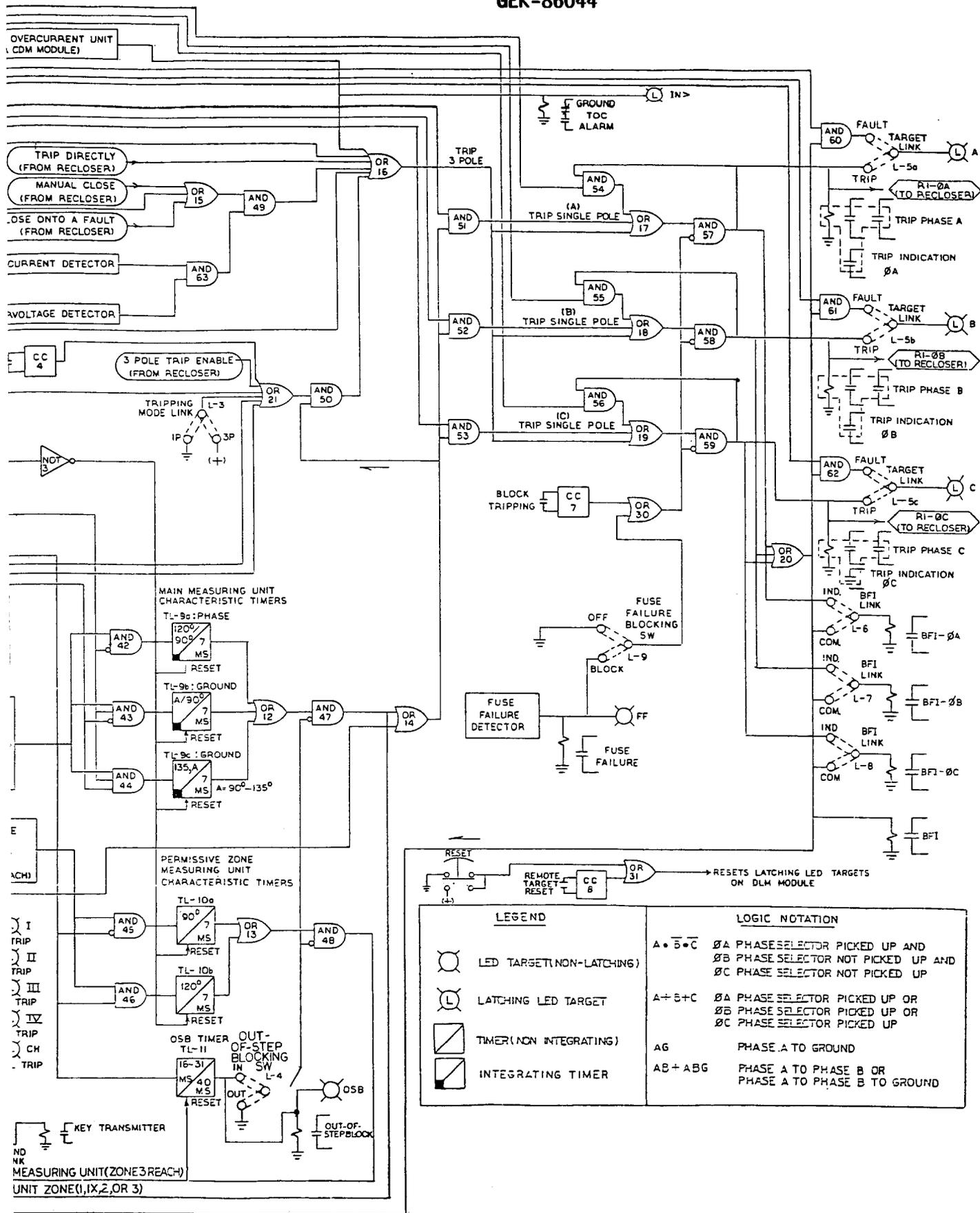
\*Figure 5 (0145D8908-5) Logic Diagram of SLS Distance Relay
