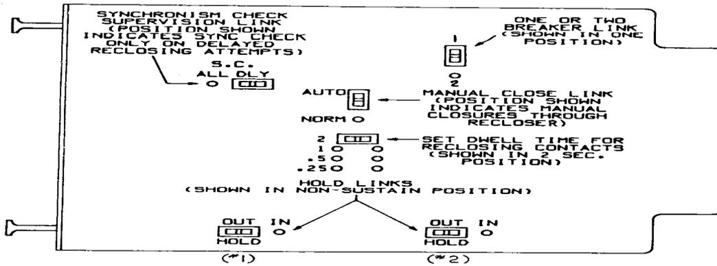
Figure 35 (0285A6623-1) Internal Links - RLM101 Module
