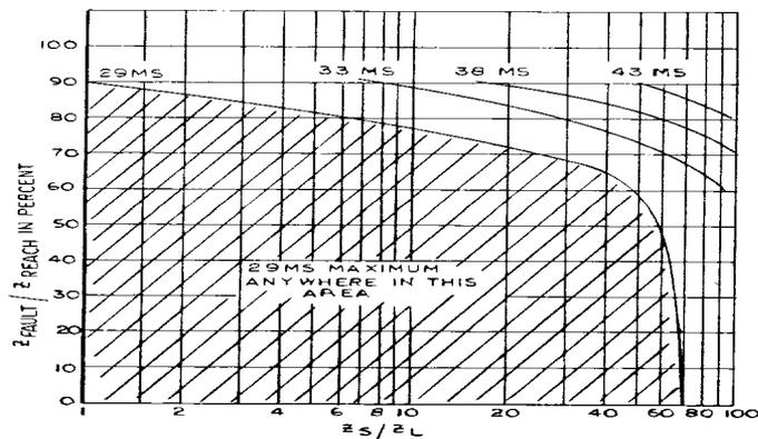
Figure 76 (0285A6684-1) Constant Time Operating Curves - Phase-to-Ground Faults (Maximum)
