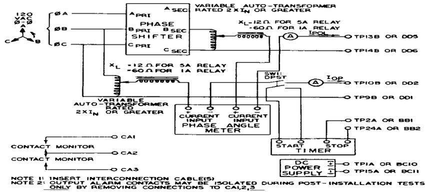
Figure 68 (0285A7568-0) Test Circuit for Directional Ground Time Overcurrent Function Using Current Polarization
