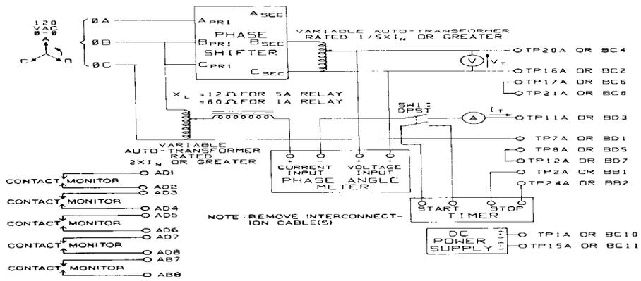
Figure 51 (0285A6611-1) Test Circuit for Zone Timer Tests
