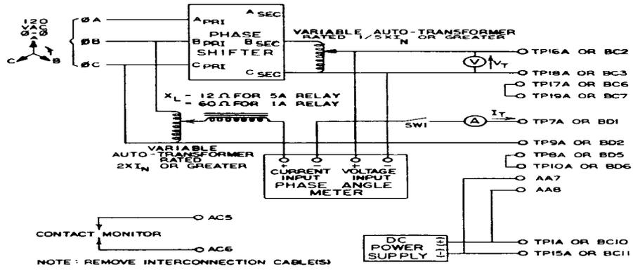
Figure 55 (0285A7573-0) Test Circuit for Out-of-Step Blocking Tests with One Pole Open
