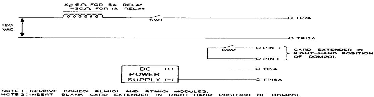
Figure 58 (0285A7583-0) Test Circuit for Post-Installation Line Pickup Test
