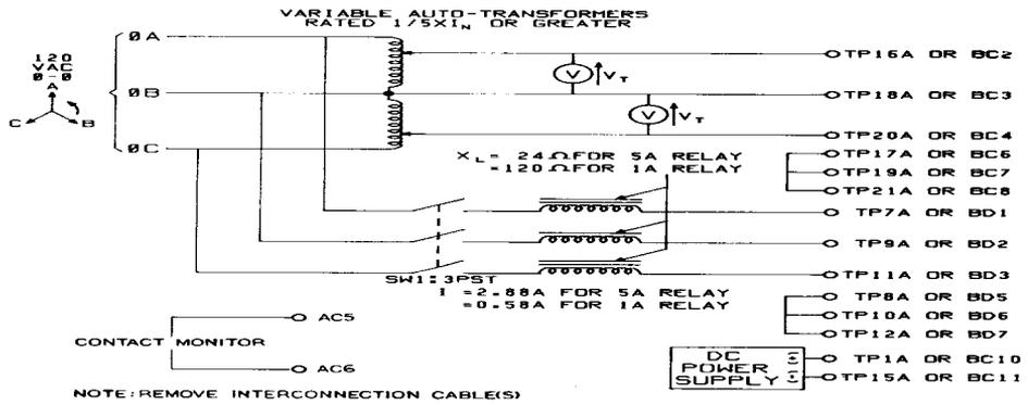
Figure 53 (0285A6612-1) Test Circuit for Out-of-Step Blocking Test
