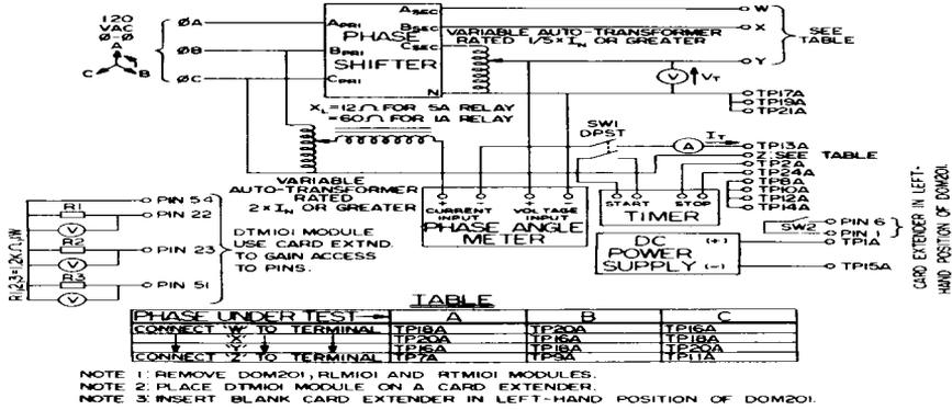
Figure 66 (0285A7571-0) Test Circuit for Post-Installation Directional Comparison Blocking and Zone 5 Tests
