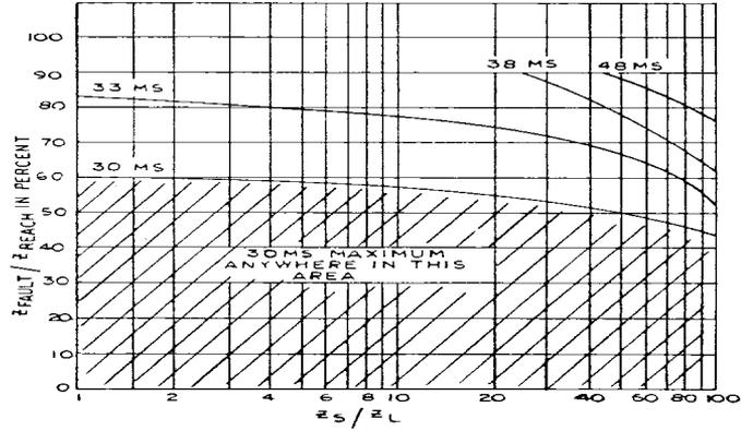
Figure 78 (0285A6686-1) Constant Time Operating Curves - Phase-to-Phase Faults (Maximum)
