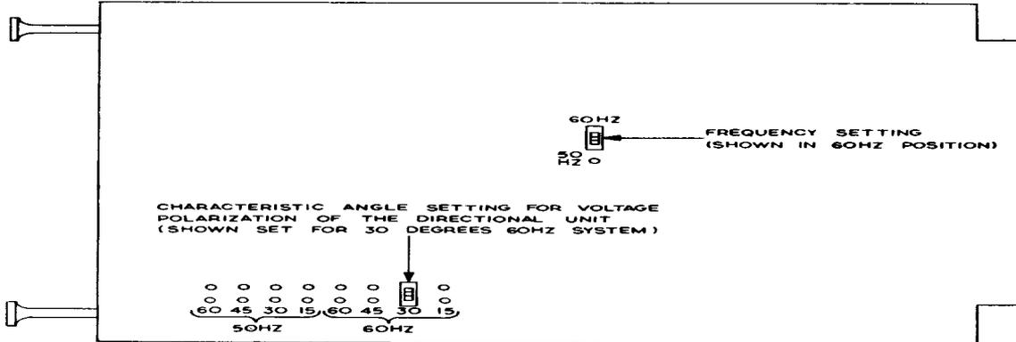
Figure 38 (0285A7563-0) Internal Links - CDM Module
