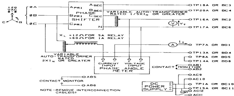
Figure 59 (0285A6613-1) Test Circuit for Testing Pilot Schemes
