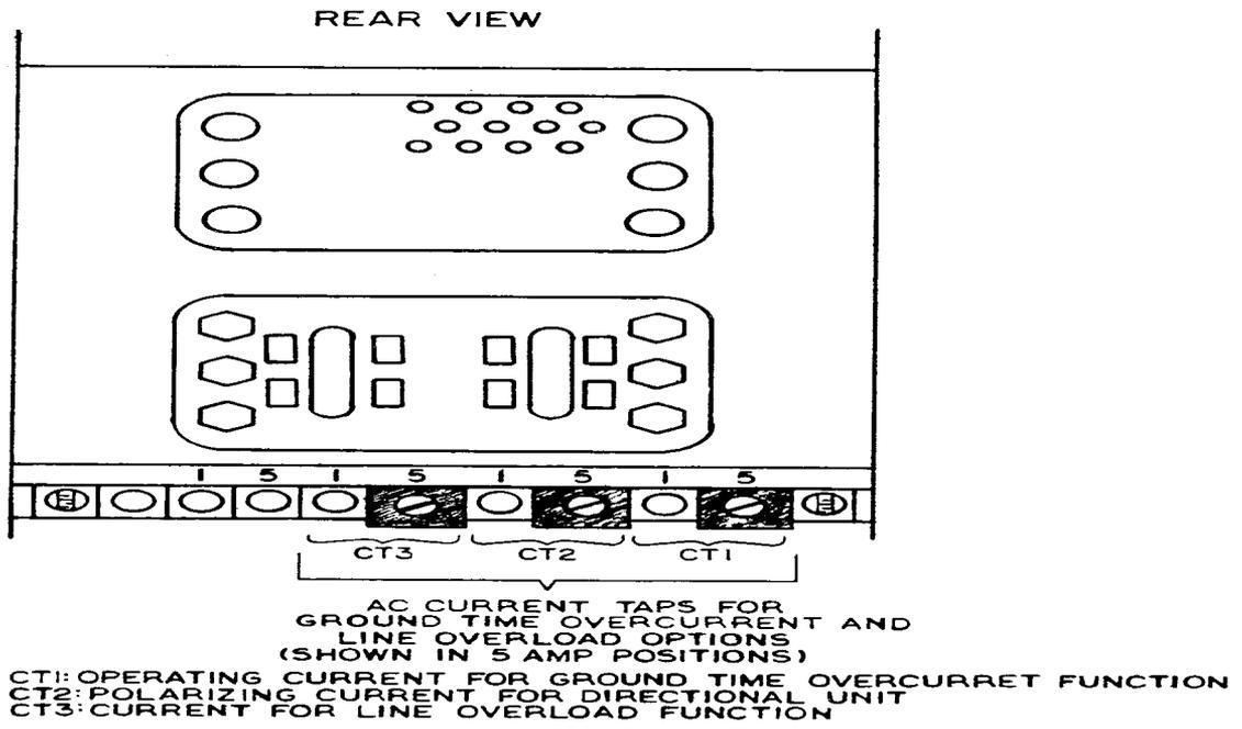
Figure 41 (0285A7560-0) Current Taps for Optional Functions In Case B MGM Module
