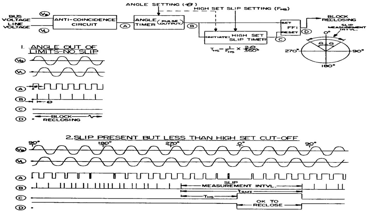
Figure 13 (0285A7549-1) SLS Angle and High Set Slip Detector
