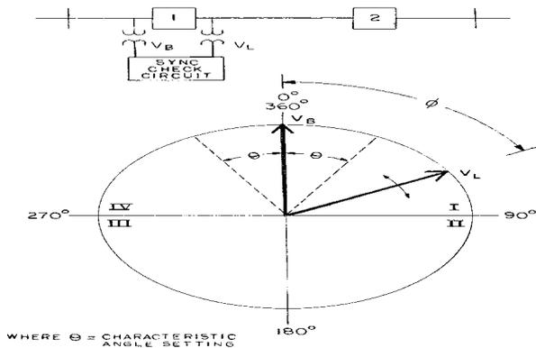
Figure 47 (0285A8201-0) System and Phasor Diagram for Synchronism Check Discussion
