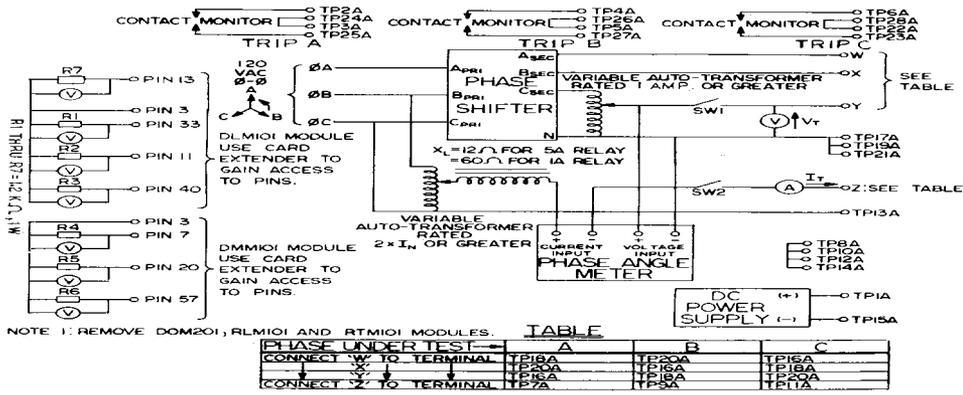
Figure 49 (0285A7574-1) Test Circuit for Post-Installation Single Phase-to-Ground Reach Tests
