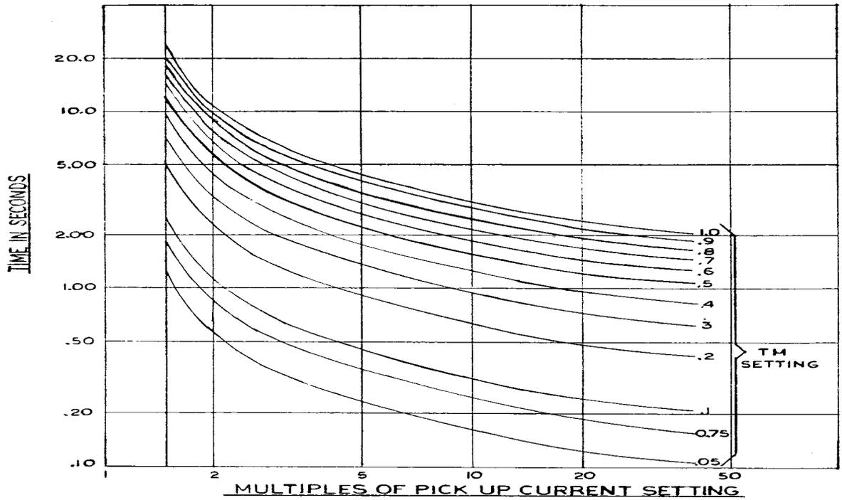
Figure 81 (0285A7557-0) Time Current Characteristics for SLS Ground Time Overcurrent Unit
