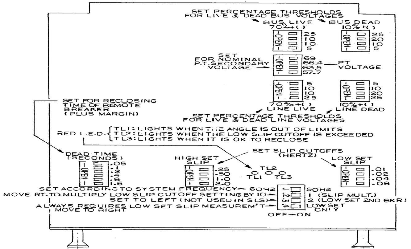
Figure 39 (0285A7564-2) Internal Switches and LEDs, SVM Module
