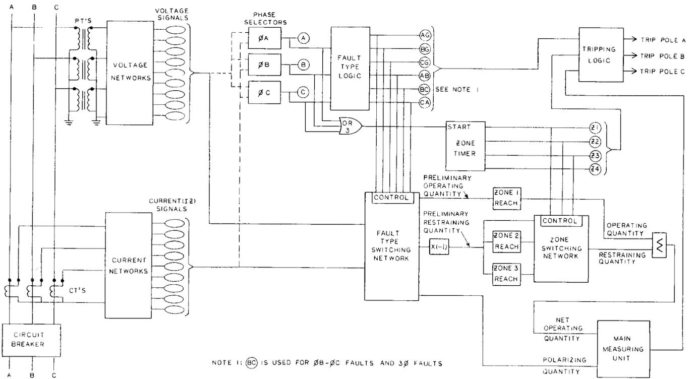
Figure 1 (0138B7648-0) Simplified Block Diagram of SLS1000 Stepped Distance Scheme
