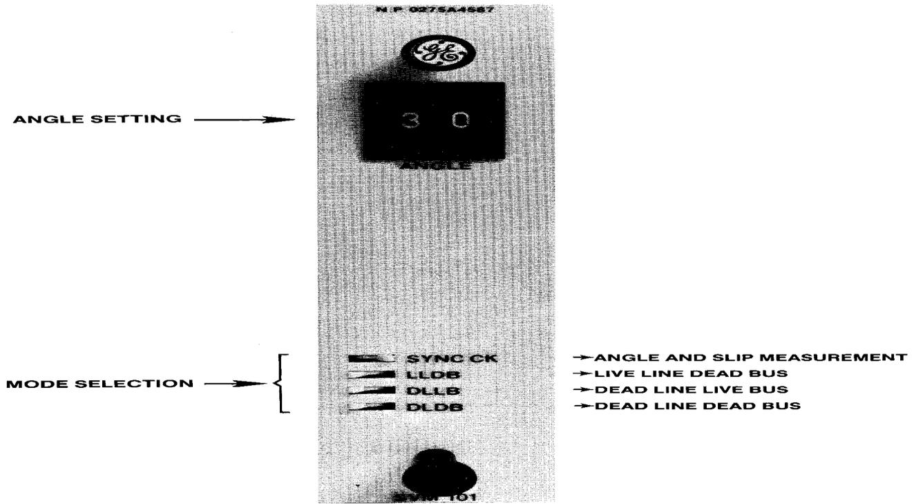
Figure 25 (8043760-0) Front View Photograph of SVM Module
