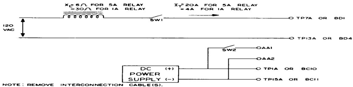
Figure 57 (0285A7584-0) Test Circuit for Line Pickup Test
