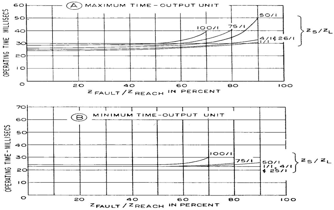
Figure 74 (0285A6681-1) Constant  $Z_S/Z_L$  Time Curves - Three Phase Faults
