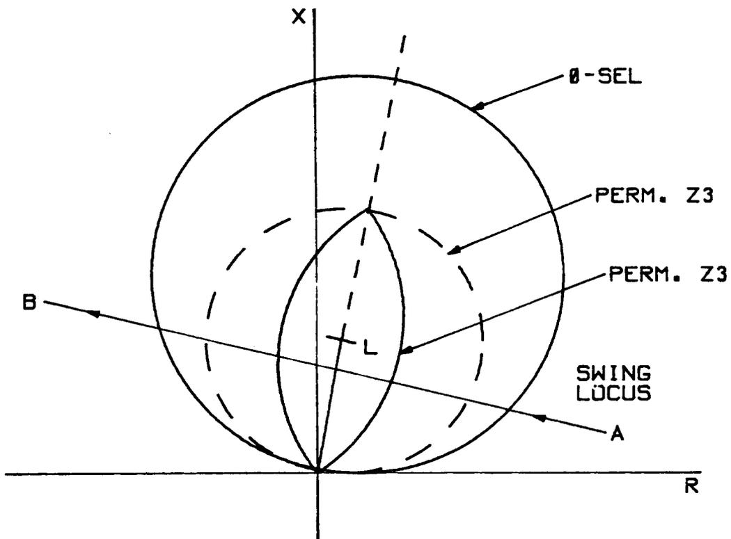
Figure 8 (0285A6630-0) Characteristics for Out-of-Step Detector Scheme
