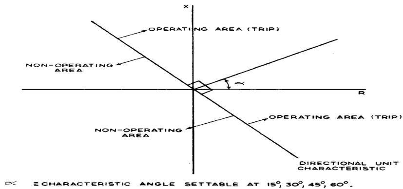
Figure 46 (0285A7553-0) R-X Characteristic for Directional Unit with Voltage Polarization
