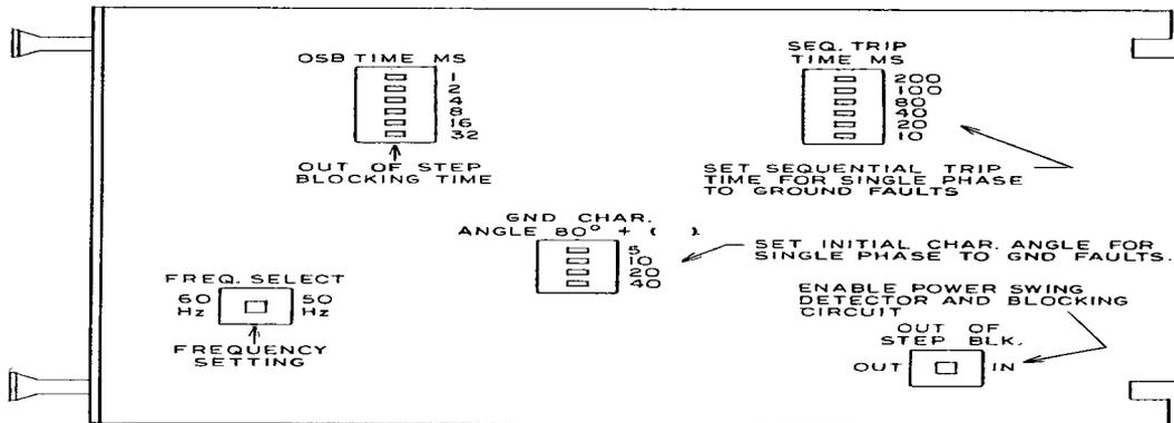
Figure 29 (0285A9109-0) Internal Links and Switches - DMM101 Module
