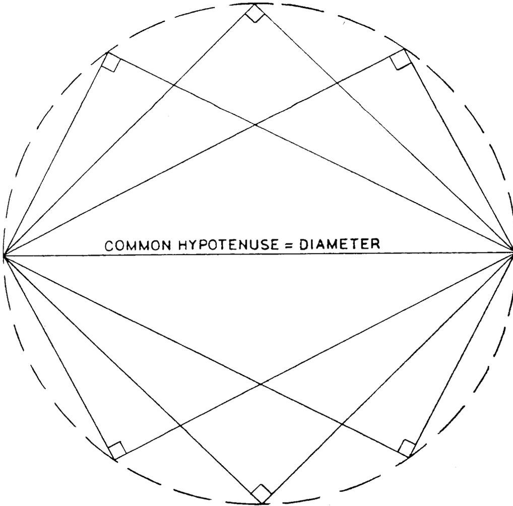
Figure 4 (0285A6689-0) Formation of a Circle by Constructing Right Triangles About a Common Hypotenuse
