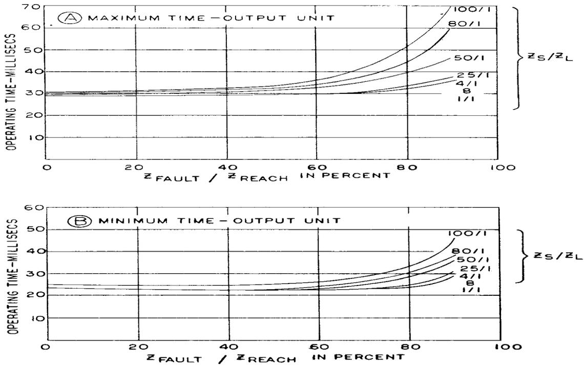
Figure 73 (0285A6683-1) Constant  $Z_S/Z_L$  Time Curves - Phase-to-Phase Faults
