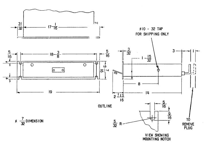
Fig. 1 (0227A2036-0) Outline and Mounting Dimensions for the SLYG62B Relay
