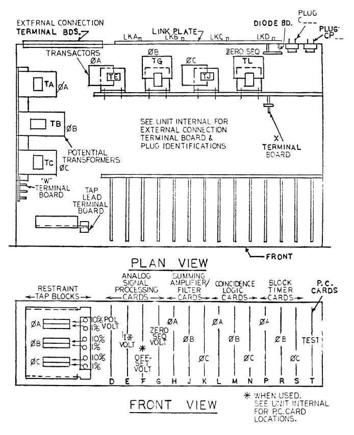
Fig. 3 (0269A3158-1) Component Location Diagram for the SLYG62B Relay
