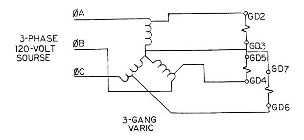
Fig. 6 (0285A6179-0) Test Circuit and Wave Form for Polarizing Sensitivity Setting
