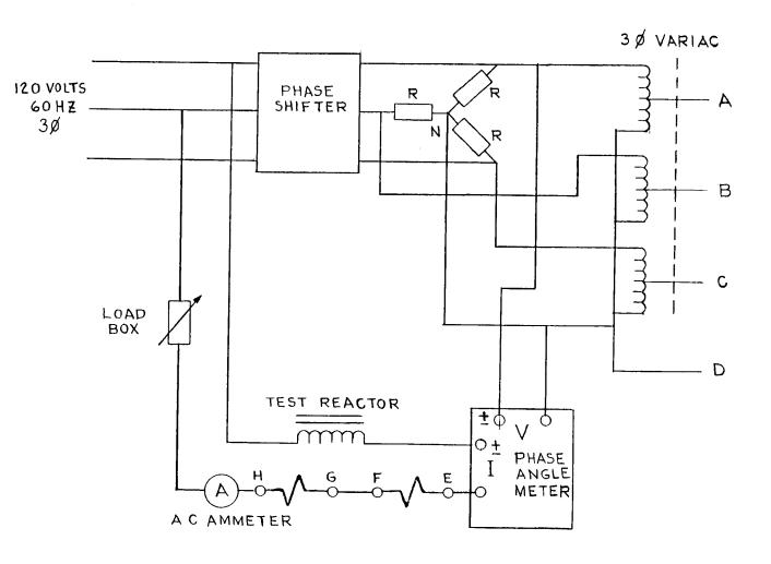
Fig. 7 (0273A9547-0) Test Circuit for Offset Characteristic Test
