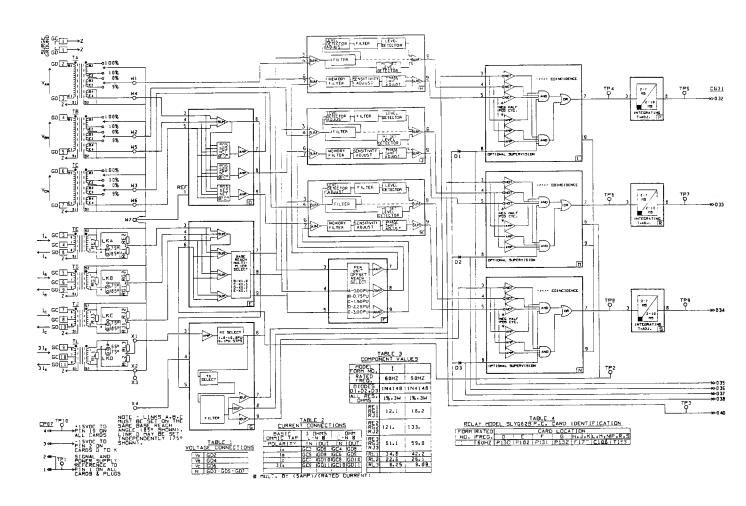
Fig. 2 (0136D5121-0) Internal Connection Diagram for the SLYG62B Relay
