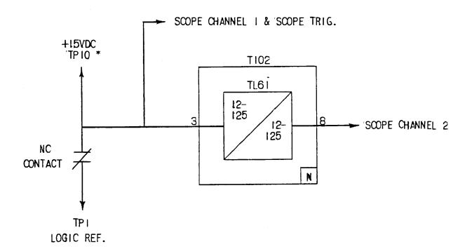
\* THE 15VDC SIGNAL AT RIN 10 HAS A CURRENT LIMITING RESISTOR MOUNTED ON THE TEST CARD.
