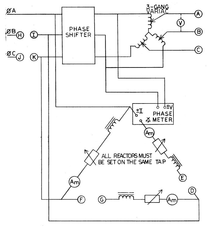
FIG. 10 (0246A6881-1) SLYN Unit Test Circuit-Method I
