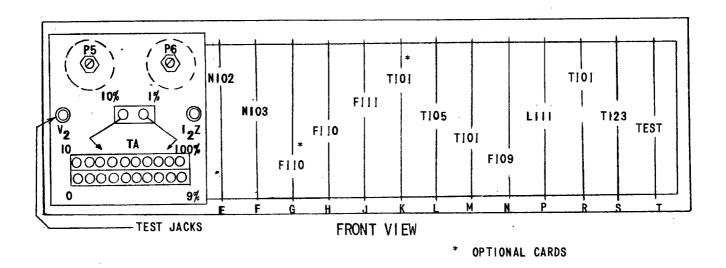
FIG. 2 (0246A2495-2) Component Location Diagram For The Type SLYN51A Relay
