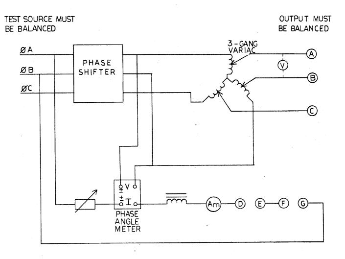
FIG. 11 (0246A6880-1) SLYN Unit Test Circuit-Method II
