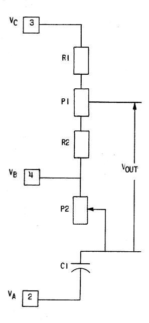
FIG. 4 (0227A2176-0) SLYN Negative Sequence Voltage Network
