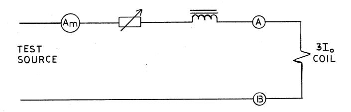
FIG. 12 (0246A6879-0) SLYN 3Io Test Circuit
