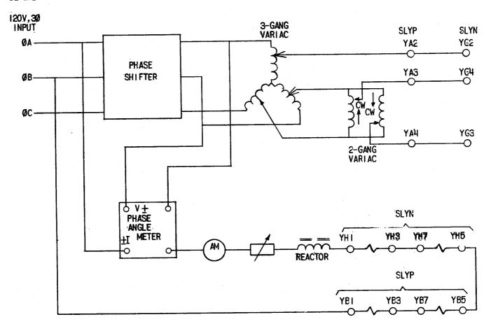
FIG. 14 (0227A2177-1) Amplitude Comparator Test Circuit
