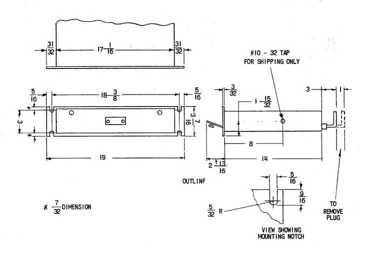
FIG. 1 (0227A2036-0) Outline And Mounting Dimensions For The Type SLYN51A Relay
