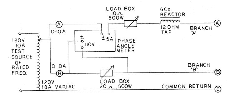
FIG. 9 (0246A6882-1) SLYN Current Network Test Connections-Method II
