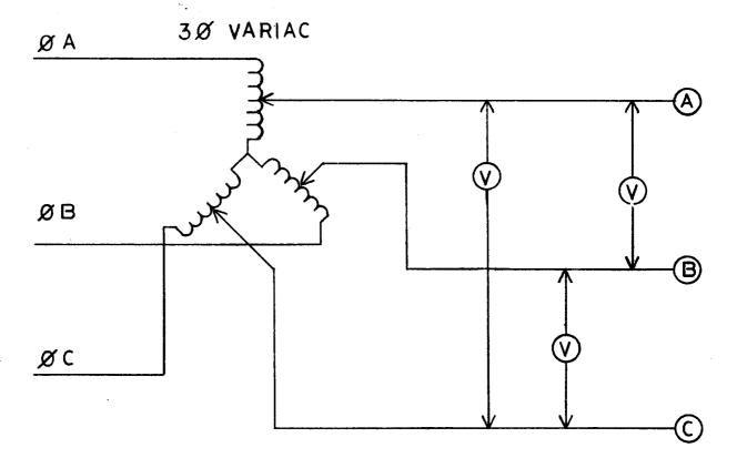
FIG. 7 (0246A6884-1) SLYN Voltage Network Test Connections
