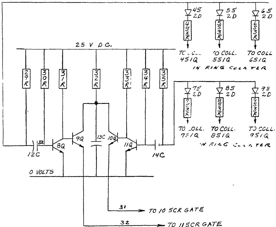
Figure 9. Gating Circuit For Commutation SCR's
