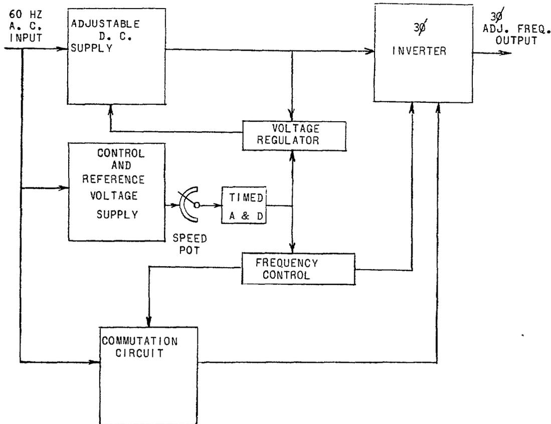
Figure 1. Power Unit Block Diagram
