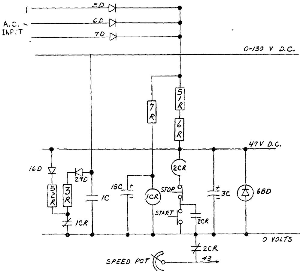
Figure 2. Start-Up Circuit
