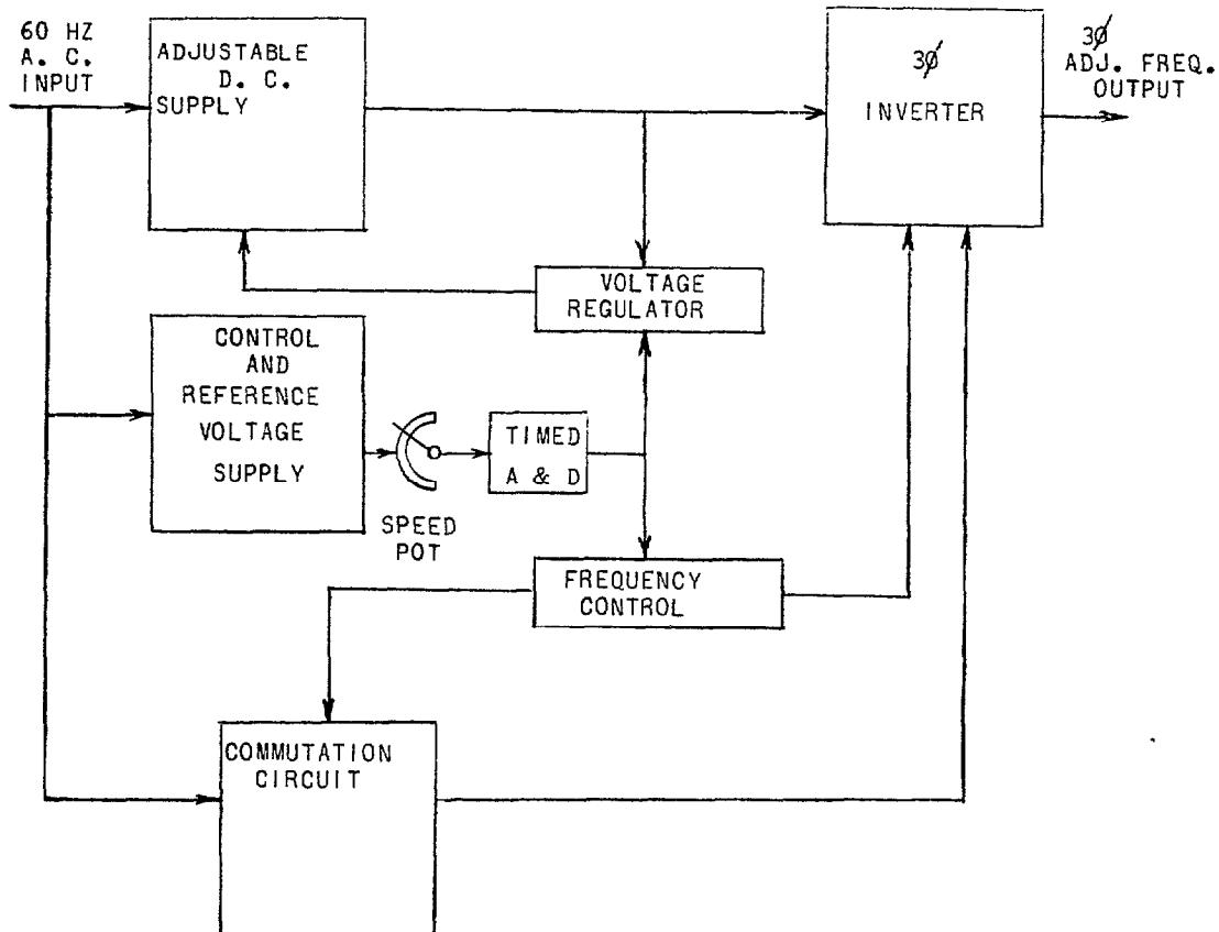
Figure 1. Power Unit Block Diagram
