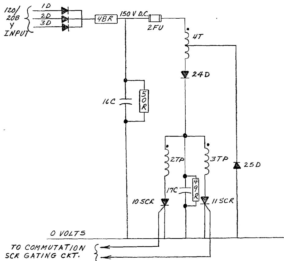
Figure 14. Commutation Circuit
