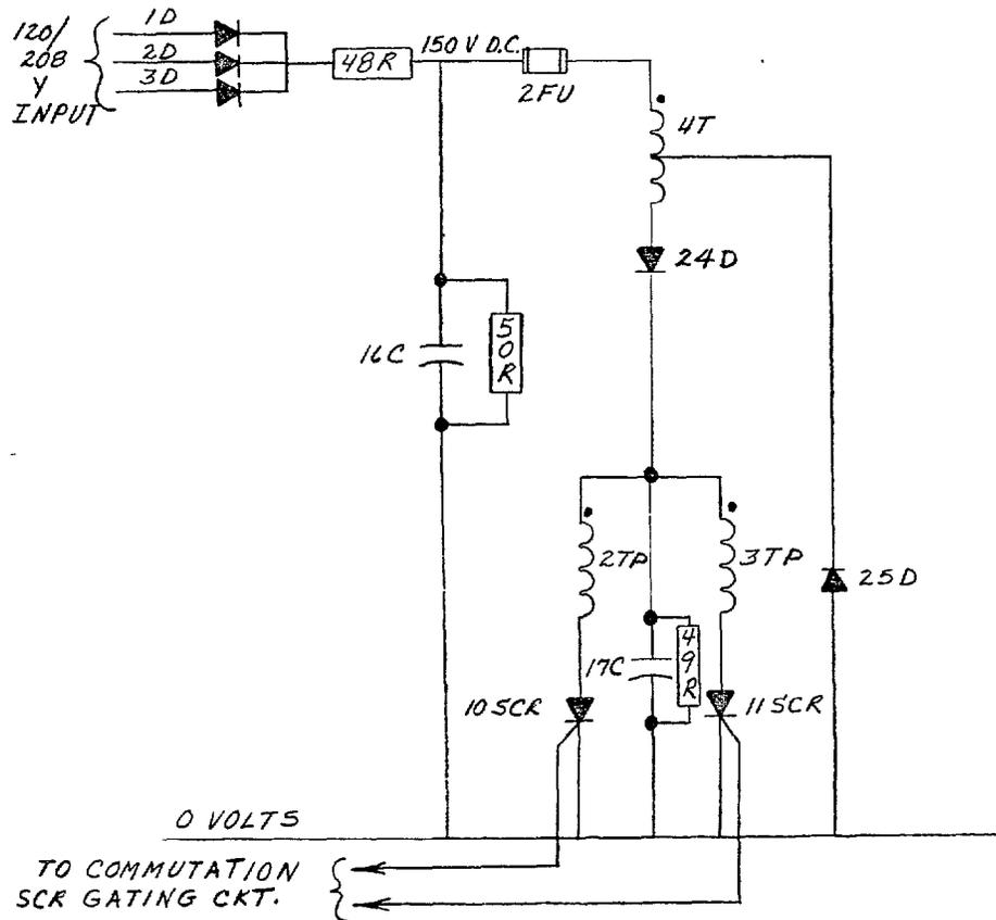
Figure 14. Commutation Circuit
