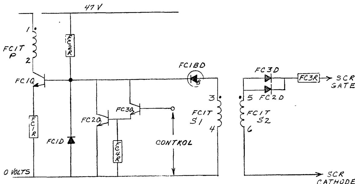
Figure 7. Firing Circuit
