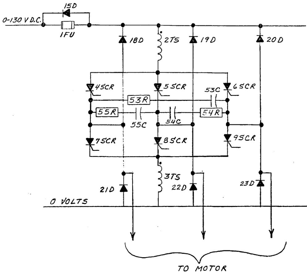
Figure 12. Inverter Bridge
