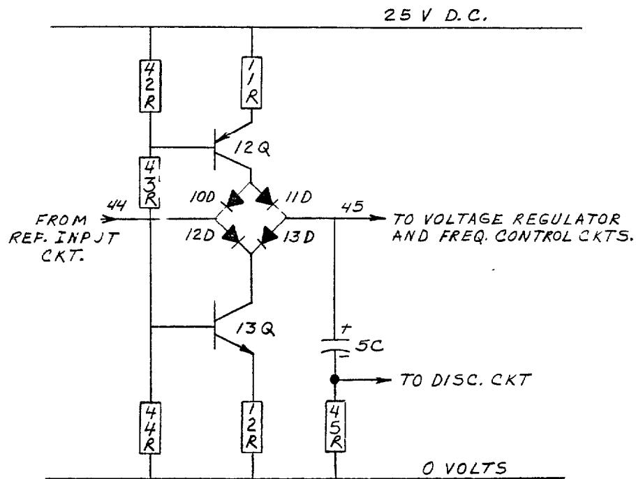
Figure 4. Timed Acceleration and Deceleration Control Circuit
