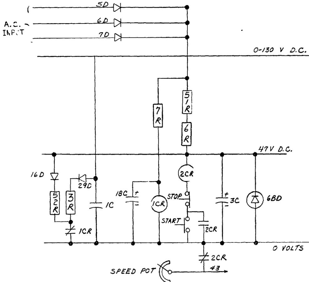
Figure 2. Start-Up Circuit
