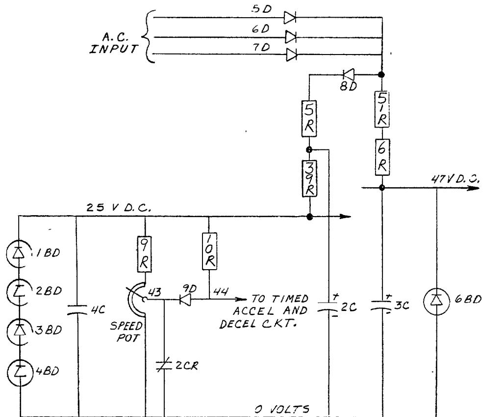
Figure 3. Control Power Supply and Reference Input Circuit
