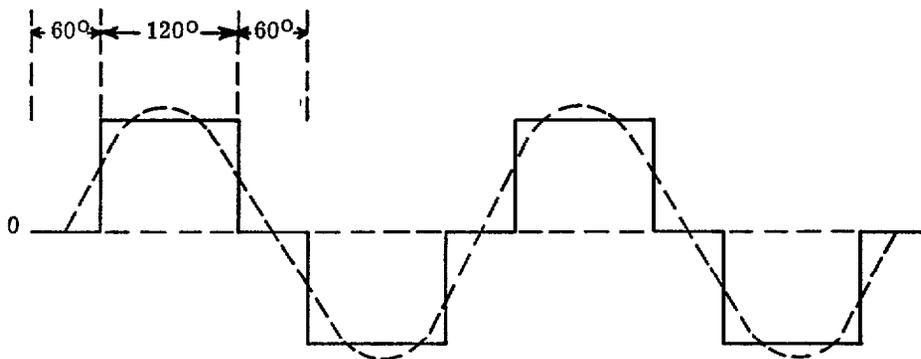
Figure 13. Inverter Output Line to Line Voltage
