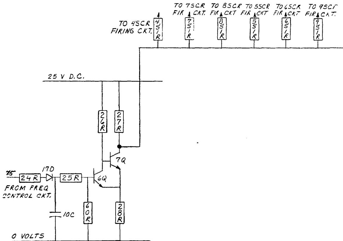
Figure 8. Blanking Circuit
