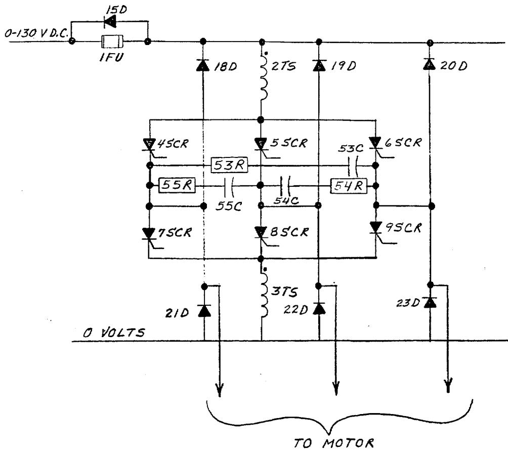
Figure 12. Inverter Bridge
