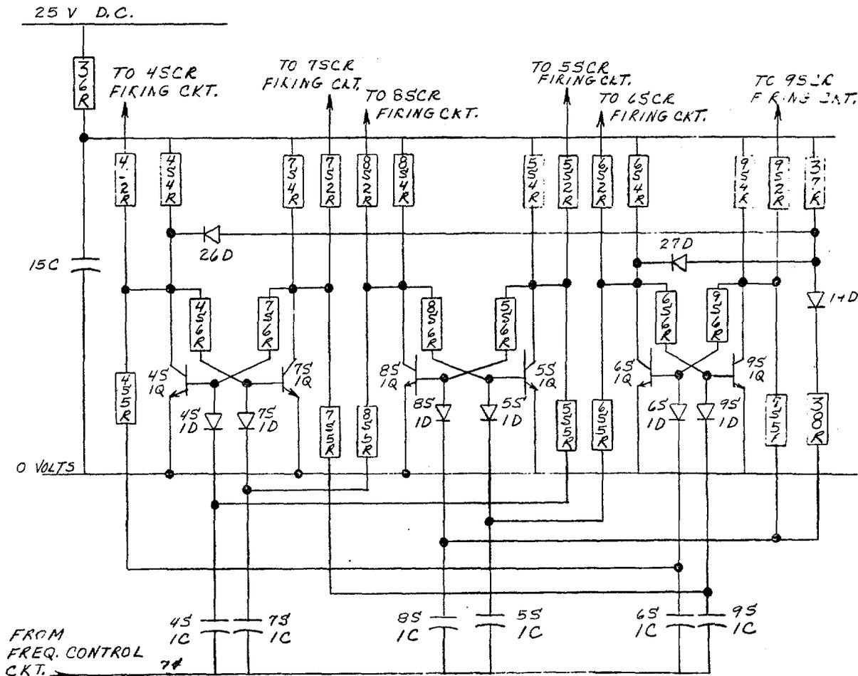
Figure 11. Ring Counter Circuit
