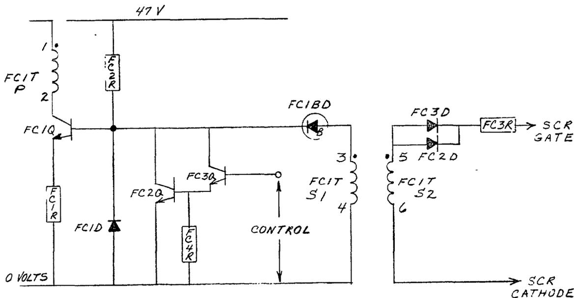
Figure 7. Firing Circuit
