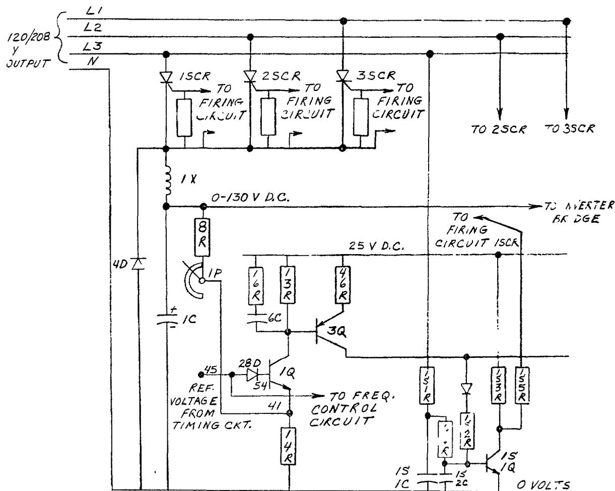
Figure 5. DC Voltage Regulator Circuit
