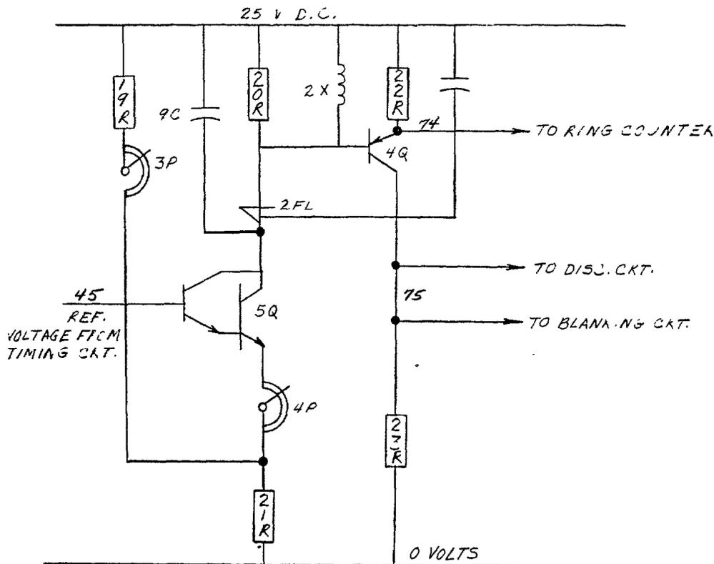
Figure 6. Frequency Control Circuit
