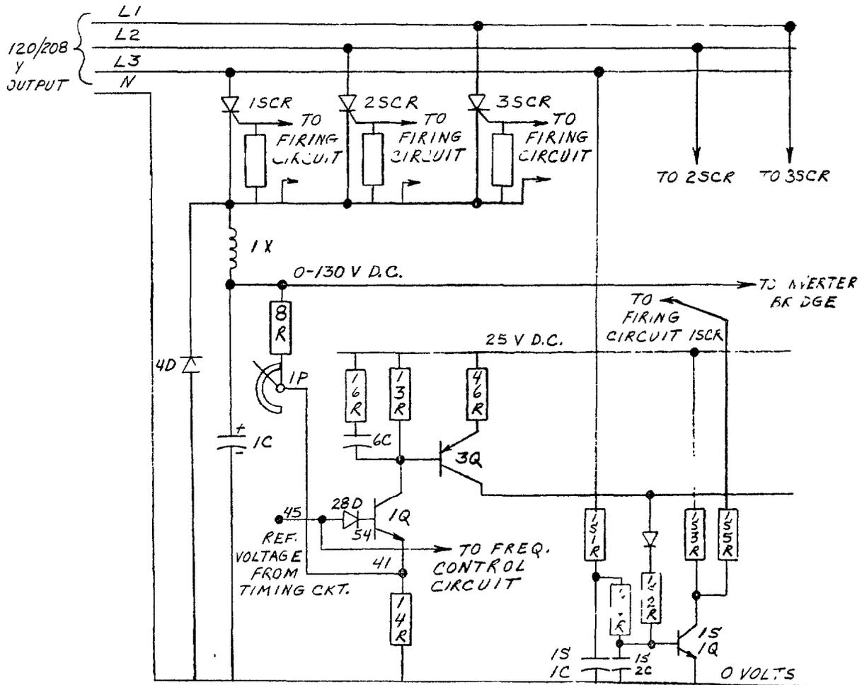
Figure 5. DC Voltage Regulator Circuit
