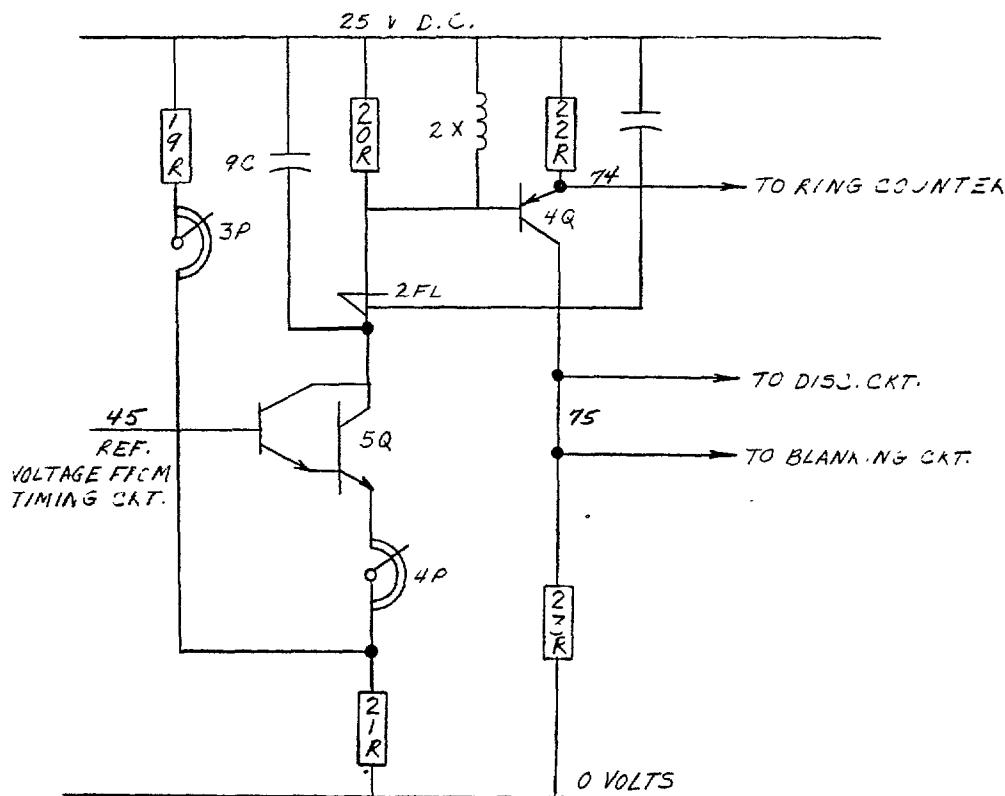
Figure 6. Frequency Control Circuit
