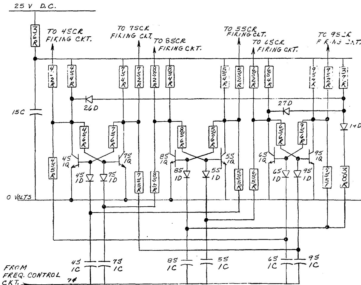
Figure 11. Ring Counter Circuit
