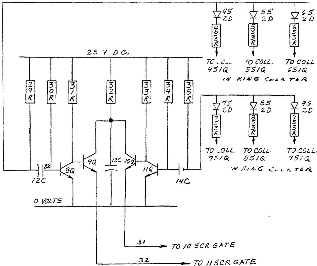
Figure 9. Gating Circuit For Commutation SCR's
