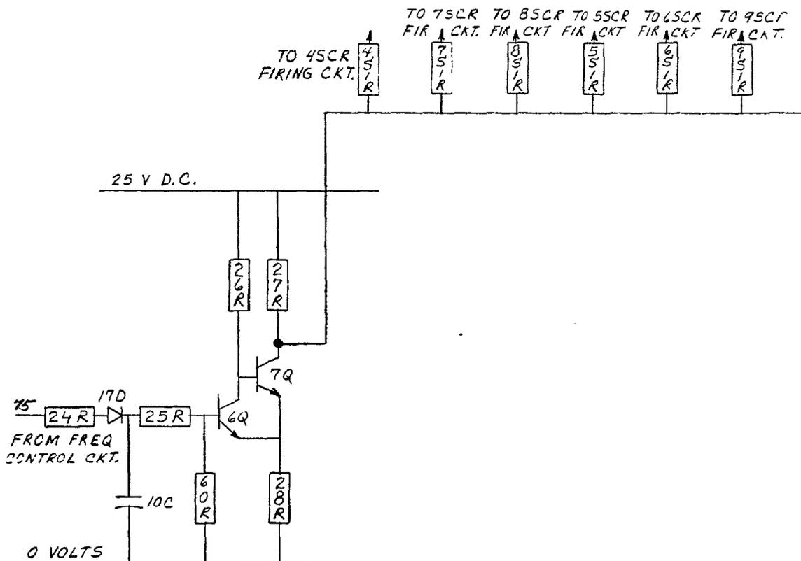
Figure 8. Blanking Circuit
