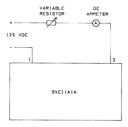
FIG. 5 ( 0257A9689-0) Test Connections for Target Unit
