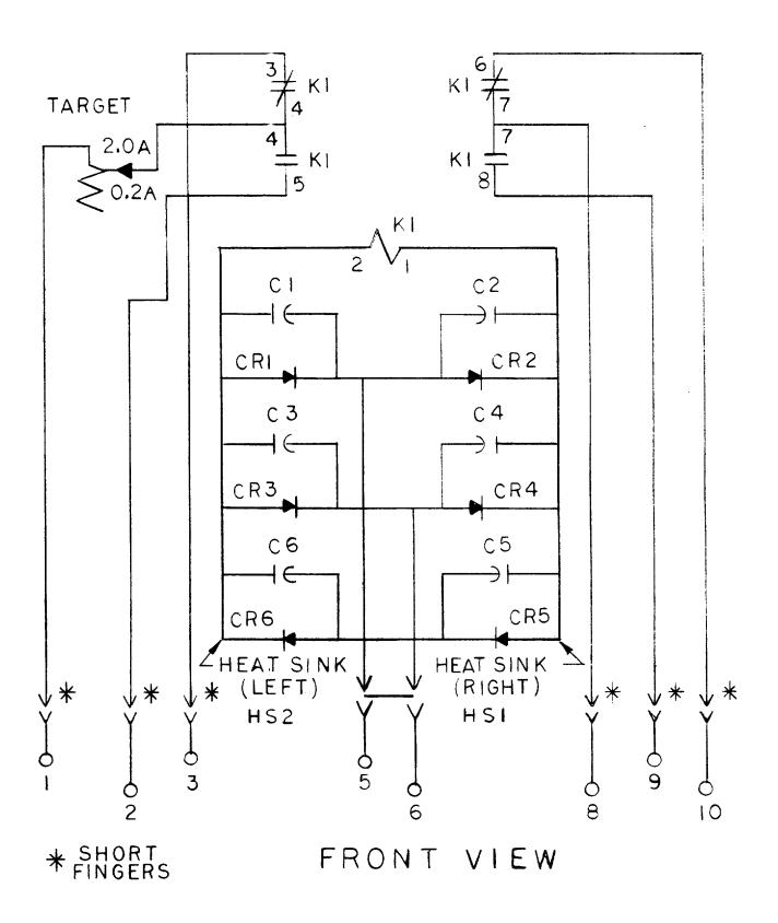
FIG. 1 (0269A3064-0) Internal Connections Diagram
