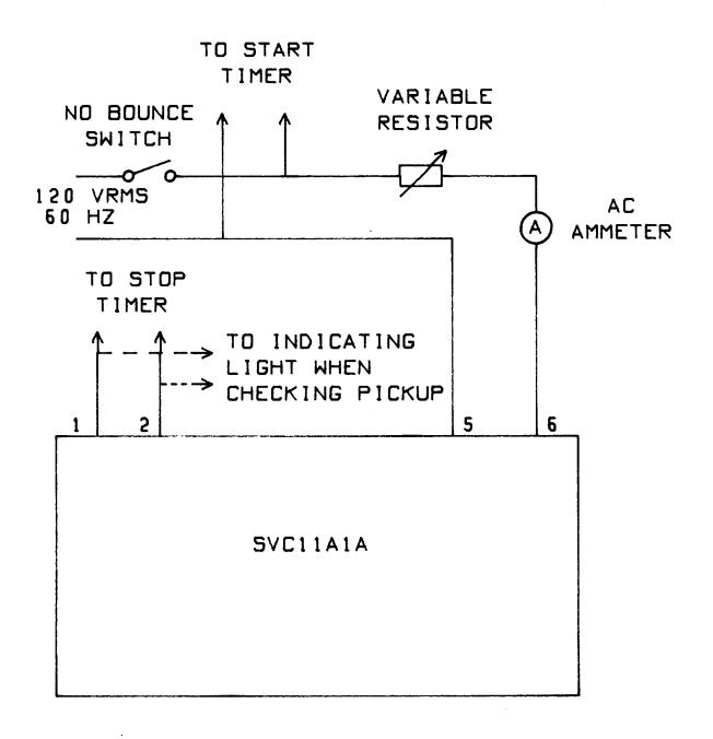
FIG. 4 ( 0257A9690-0) Test Connections for Pickup Level and Operating Time
