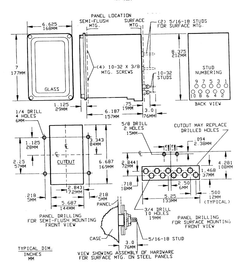
Figure 8 (0246A7968 [4]) V1 Case Outline and Panel Drilling Dimensions
