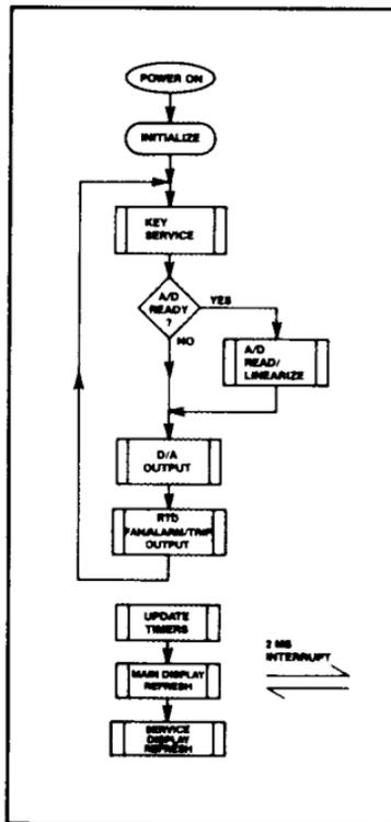
A block diagram of the firmware execution is shown in fig. 5.2. Firmware is stored in a 4K x 8 bit EPROM memory. At power on RAM memory is cleared, the real-time clock is started and parameters are initialized. Every 2 mS the clock generates an interrupt to update the timers, refresh the front panel display and read the keyboard. A service display which can be connected for calibration and diagnostic use is also refreshed at this time.
