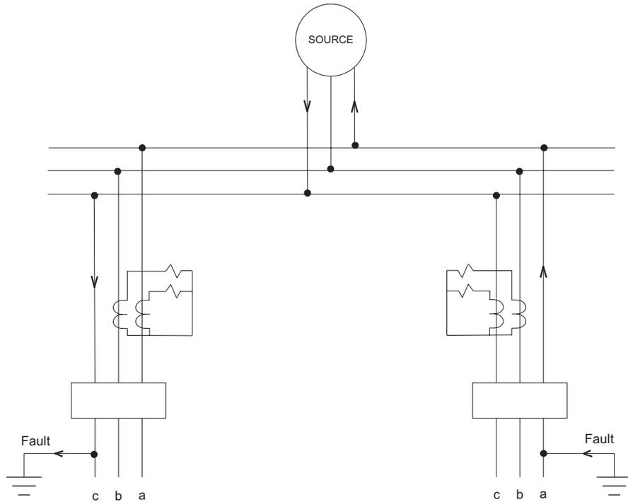
**FIGURE 1. Lack of Protection with Two Overcurrent Elements**
