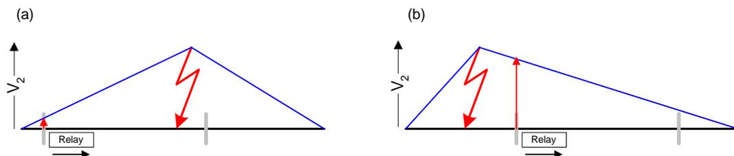
Figure 17. Polarizing voltage could be low during forward faults (a), but is typically high for reverse faults (b).
