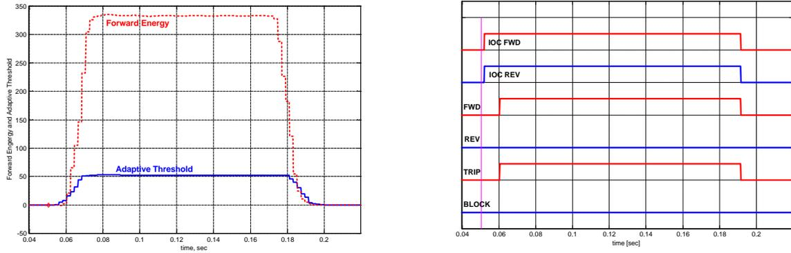
Figure 21. Sample double-line-to-ground fault: Negative-Sequence Forward and Restraining Energies (left); Negative-Sequence Logic Flags (right). The forward-looking element operates in 10 msec.
