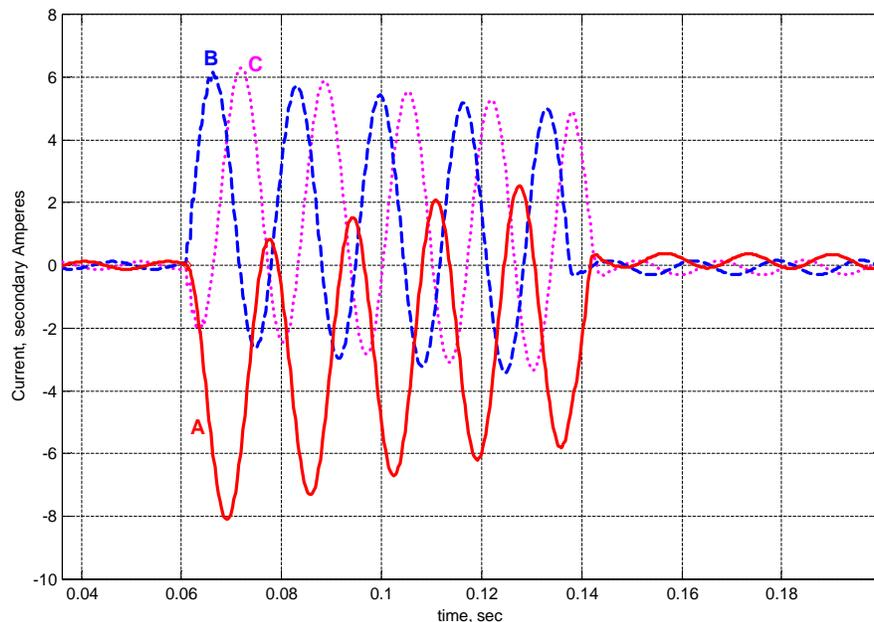
Figure 2. Sample three-phase symmetrical fault: Current Waveforms. The three phase currents develop from the same pre-fault magnitudes to the same fault magnitudes, but the transition takes place at different initial (fault inception) angles.
