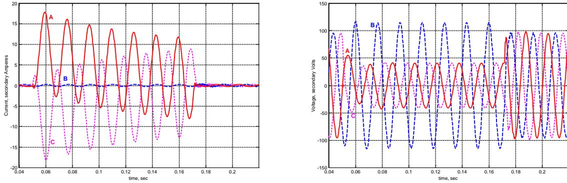
Figure 20. Sample forward double-line-to-ground fault: Current (left) and Voltage (right) Waveforms.
