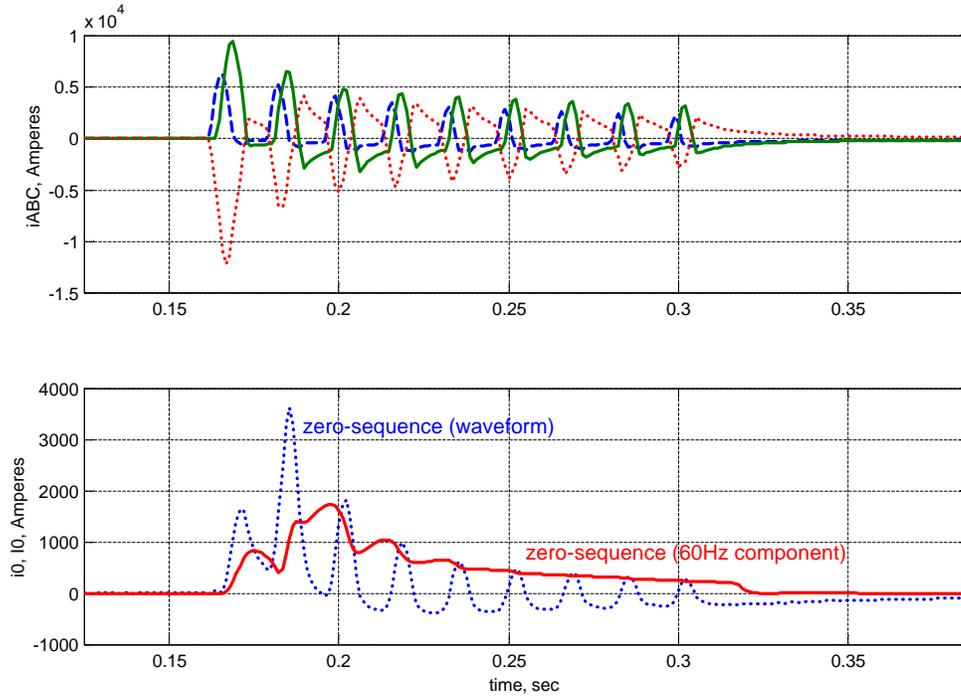
Figure 10. Sample transformer inrush currents. The transformer is energized from its delta winding – no zero-sequence expected. Due to CT saturation (long lasting dc components) spurious zero-sequence current as high as 30% of the inrush current appears.
