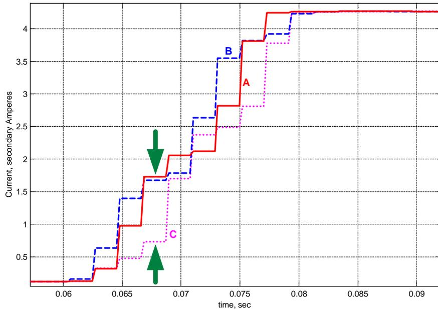
Figure 5. Sample three-phase symmetrical fault: Current Magnitudes. At 6 msec into the fault the magnitude of the phase C current substantially differs from the two other phases.
