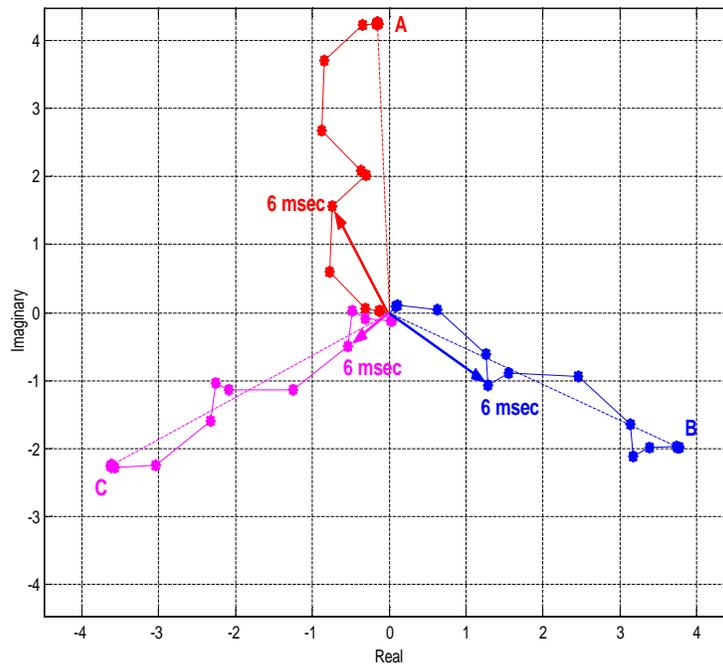
Figure 6. Sample three-phase symmetrical fault: Current ABC Phasors. The dots stand for “protection passes” being 2 msec apart. At 6 msec into the fault the ABC current diagram is unquestionably not symmetrical (the magnitudes are not equal – Fig.5, the phase angles are not 120 degrees apart – Fig.4).
