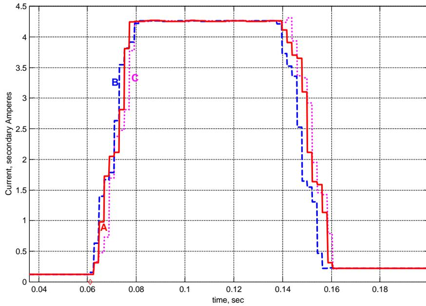
Figure 3. Sample three-phase symmetrical fault: Current Magnitudes. Due to different fault inception angles the three phase currents ramp up (and down when the fault gets cleared) in slightly different ways.
