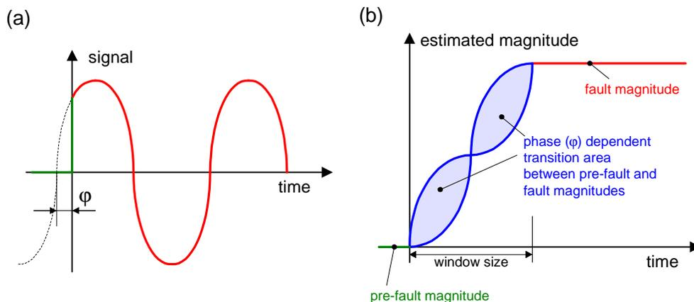
Figure 1. Initial phase angle of the signal developing from a pre-fault magnitude to a fault magnitude (a) causes uncertainty of the transition from the pre-fault to fault values of the estimated signal magnitude (b).
