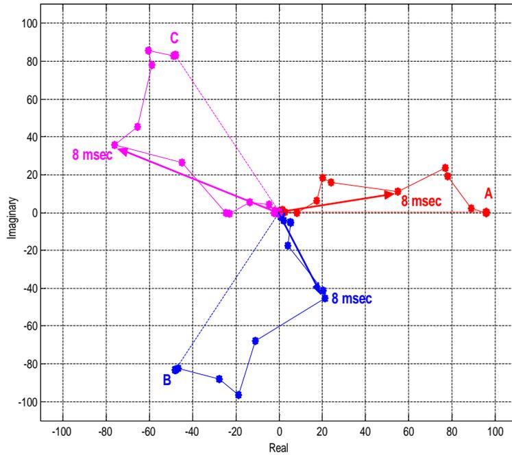
Figure 13. Sample three-phase symmetrical fault: Voltage ABC Phasors. At 8 msec into the fault the ABC voltage diagram is unquestionably not symmetrical.
