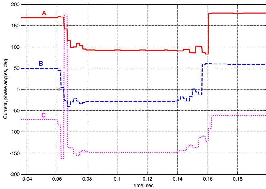
Figure 4. Sample three-phase symmetrical fault: Current Phase Angles. Due to different fault inception angles the three phase currents change their phase angles in slightly different ways.
