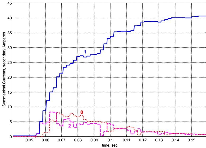
Figure 9. Sample symmetrical fault with heavy CT saturation: Current Symmetrical Components (012). Due to CT saturation spurious negative- and zero-sequence currents appear for considerable time.
