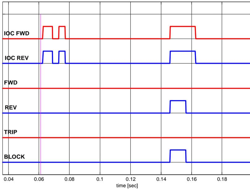
Figure 19. Sample three-phase symmetrical fault: Negative-Sequence Logic Flags. Neither forward nor reverse looking elements operates on fault inception. Short blocking pulse appears on fault clearing.
