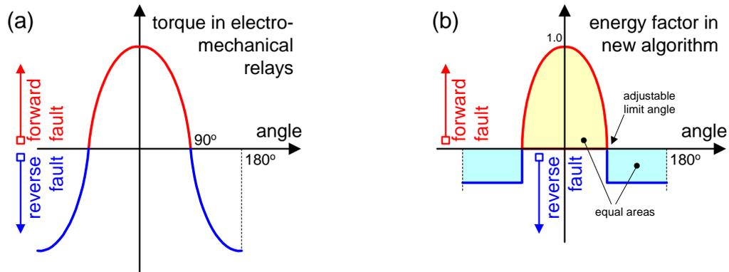
Figure 16. Electro-mechanical relays (a) vs. the new digital approach (b).
