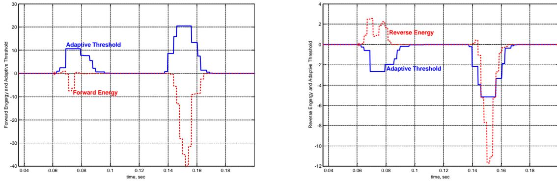
Figure 18. Sample three-phase symmetrical fault: Negative-Sequence Forward and Restraining (Adaptive Threshold) Energies (left); Negative-Sequence Reverse and Restraining Energies (right);
