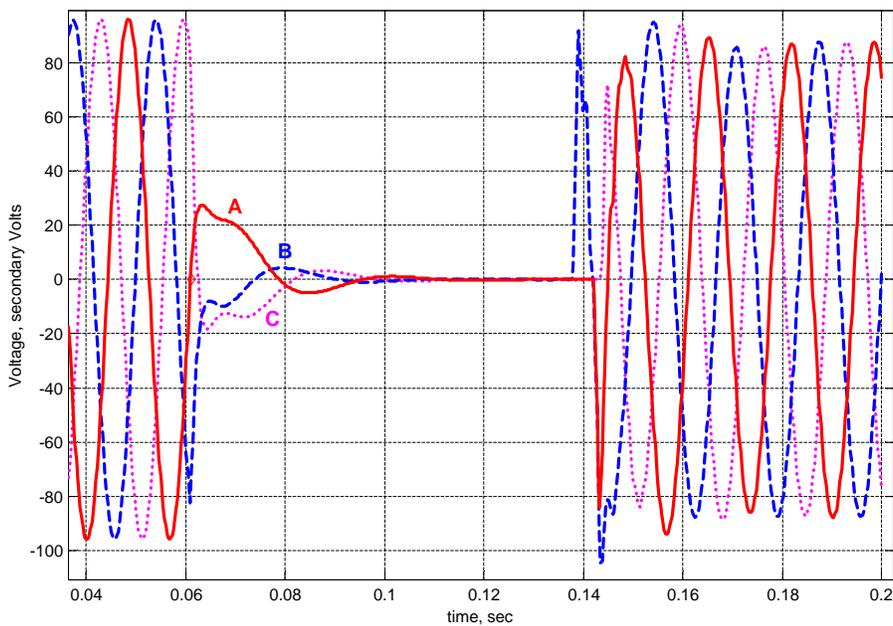
Figure 11. Sample (see Fig.2 for currents) three-phase symmetrical fault: Voltage Waveforms. Due to heavy CVT transients, the three phase voltages behave differently during first 40 msec into the fault.
