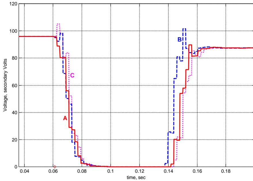
Figure 12. Sample three-phase symmetrical fault: Voltage Magnitudes.
