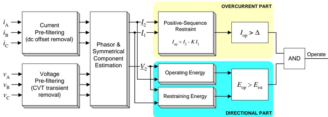
Figure 15. Simplified block diagram of the new algorithm (negative sequence shown).
