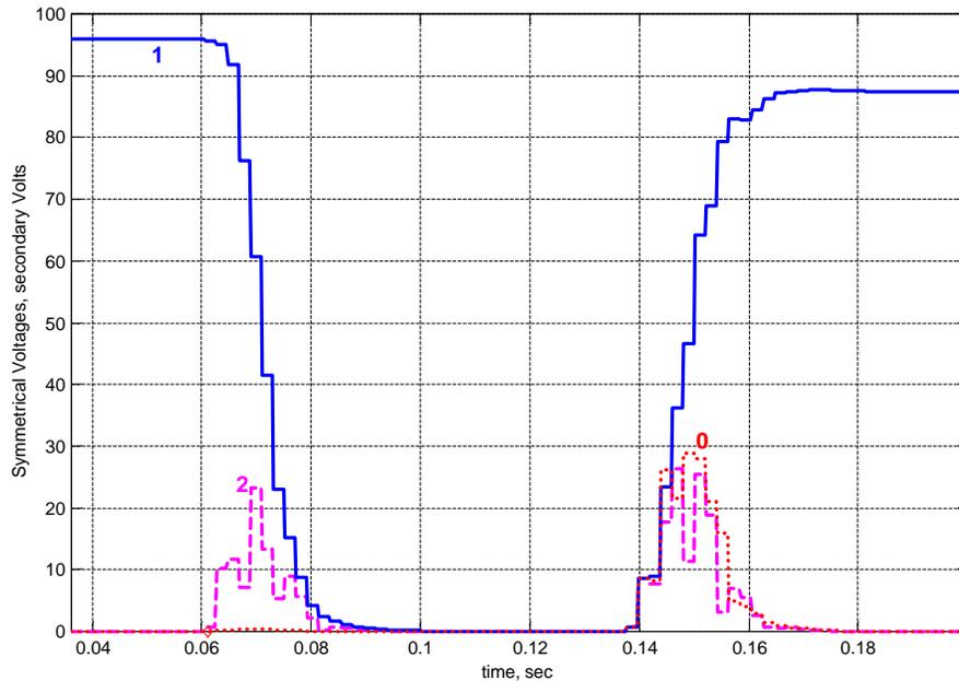
Figure 14. Sample three-phase symmetrical fault: Voltage Symmetrical Components (012).
