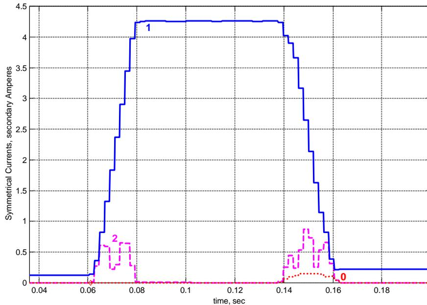
Figure 7. Sample three-phase symmetrical fault: Current Symmetrical Components (012).
