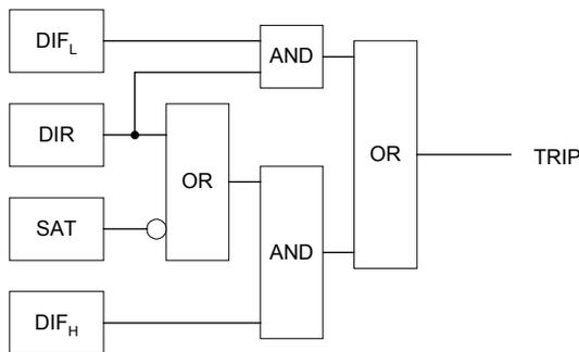
Fig.7. Adaptive trip logic.
