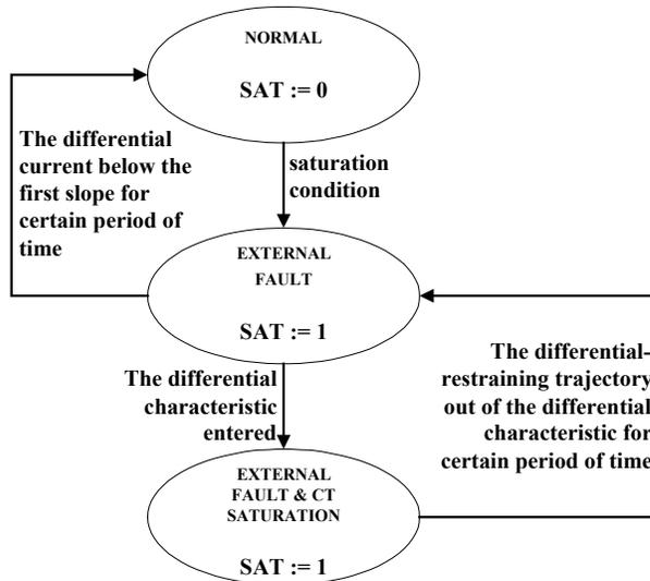
Fig.11. CT saturation detector: the state machine.
