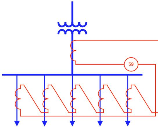
Fig.3. Busbar protection with linear couplers.
