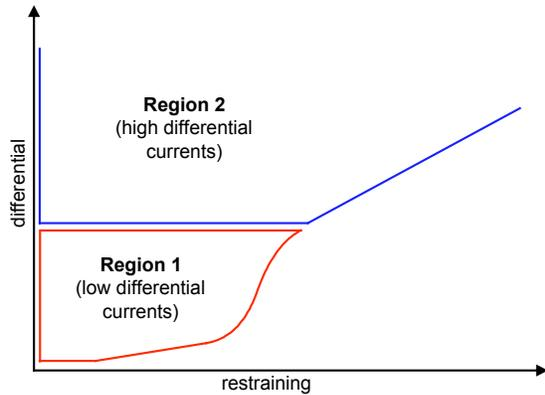
Fig.6. Two regions of the differential characteristic.
