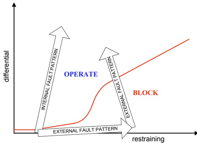
Fig.10. Saturation detection: internal and external fault patterns.
