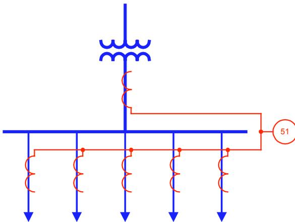
Fig.2. Overcurrent differential protection.
