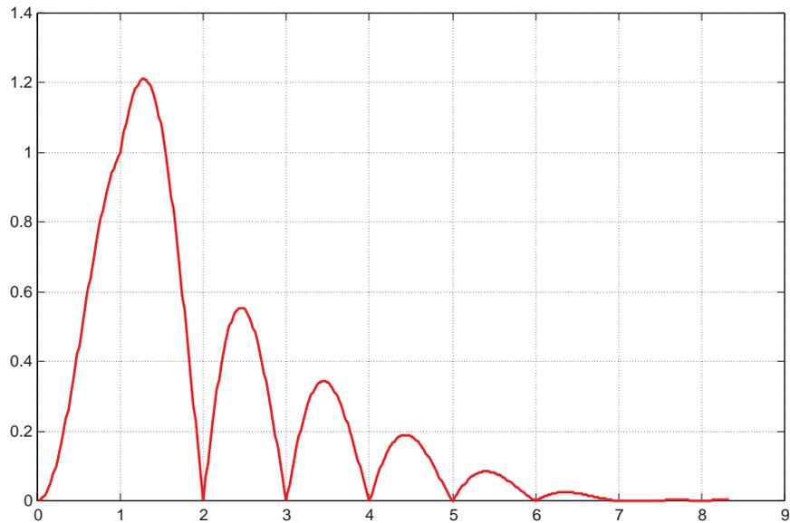
**FIGURE 1. Frequency response of the UR phasor estimator for current signals**
