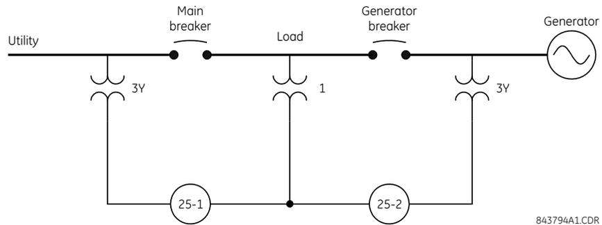
The traditional solution for either of these applications requires the use of two independent synchrocheck relays. The UR family of protection relays from GE Multilin provide two independent synchronism check functions in each relay. An individual UR-series device can have multiple voltage inputs to measure the synchronism voltages. Configurable analog signal sources allow any voltage measurement to be explicitly assigned to the two independent synchrocheck functions.
