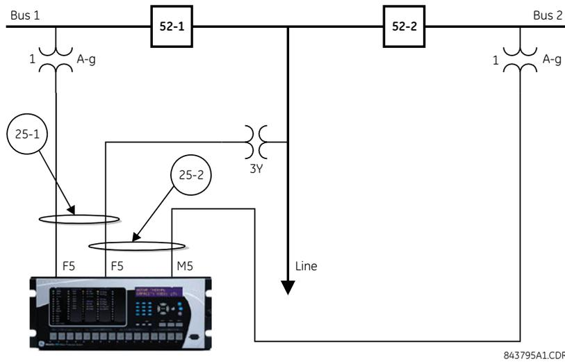
The following steps are used to configure a UR-series device to synchronize across multiple buses.
