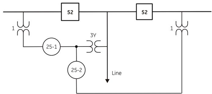
A second application is a small generation system that can operate in parallel with the utility source, or serve and maintain load separate from the utility source. In this application, it is typical to synchronize voltages across the load bus. This method requires synchrocheck from the generator to the load bus, and from the utility source to the load bus. Both synchrocheck functions use a common voltage measurement from the load bus.
