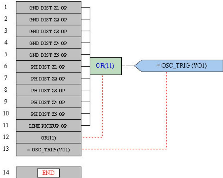
These diagrams show the FlexLogic™ equation as seen in EnerVista UR Setup.
