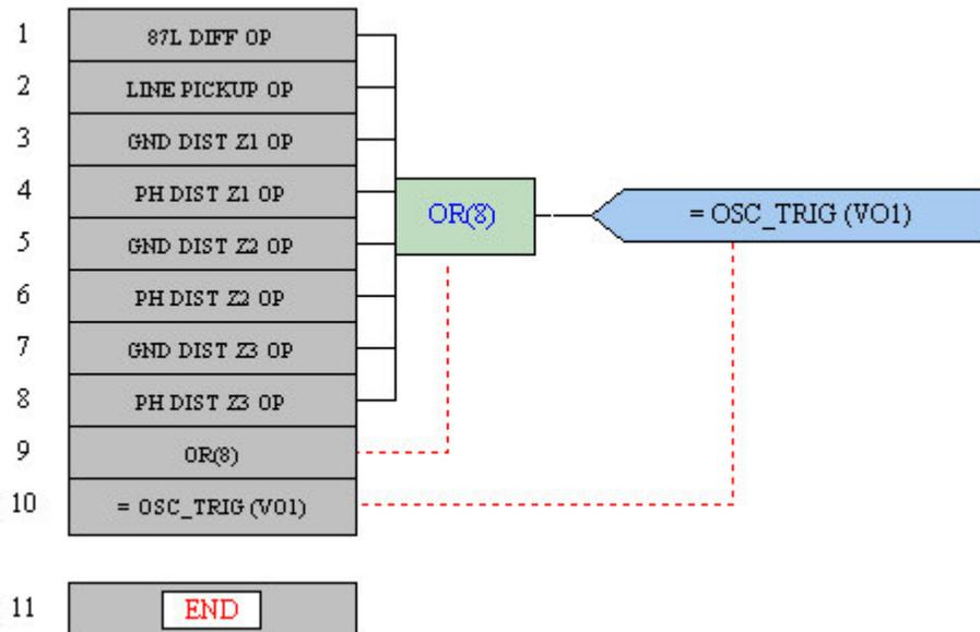
These diagrams show the FlexLogic™ equation as seen in EnerVista UR Setup.
