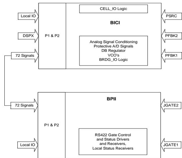
Figure 1. BICI Board and BPII Board Interface Connections
