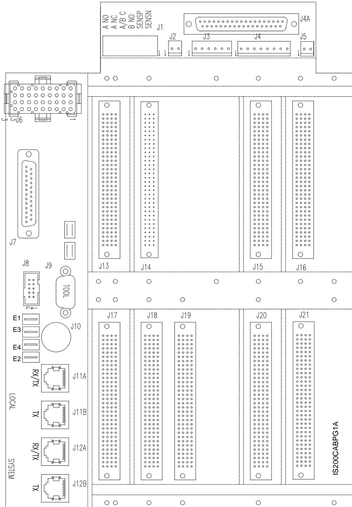
Figure 2. CABP Board Layout Diagram
