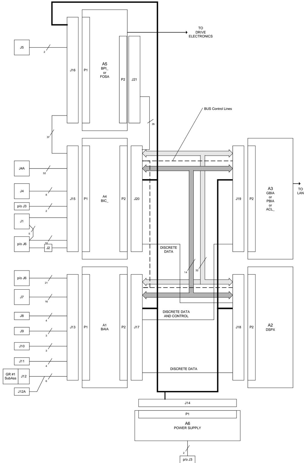
Figure 1. CABP Board Block Diagram
