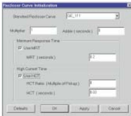
Figure 5–17: COMPOSITE RECLOSER CURVE WITH HCT ENABLED
