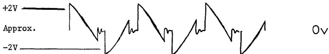
TDS e. Connect the VOM to measure  $-127V \pm 7V$  between PTB (DC1 and DC2) and with the scope monitoring "ARM V" test ring, slowly turn the TRP fully CCW and verify that the VOM indicates  $-127V \pm 7V$  and the scope display is as indicated below: Scope set at 5V/CM, 2 millise./CM.
