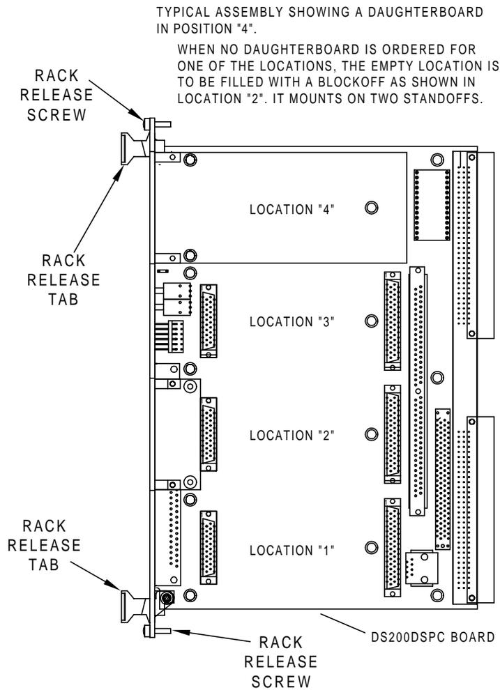
Figure 4. DSPC Board Daughterboard and Blockoff Assemblies
