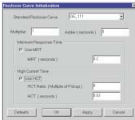
Figure 5–16: COMPOSITE RECLOSER CURVE WITH HCT ENABLED
