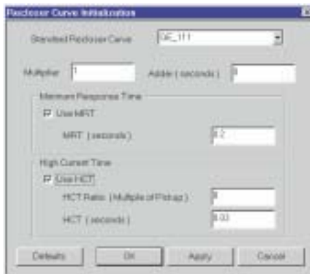
Figure 5–17: COMPOSITE RECLOSER CURVE WITH HCT ENABLED
