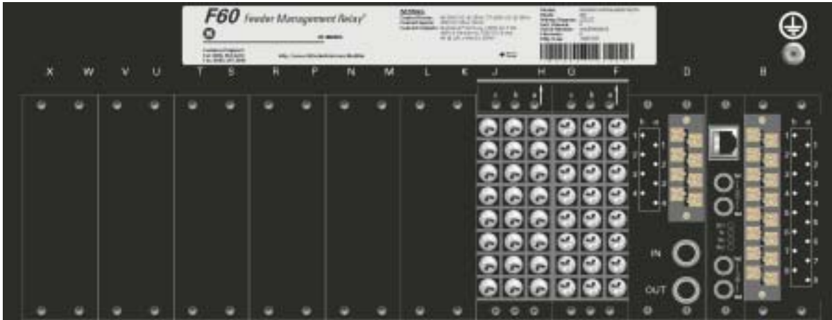
Figure 3–6: REAR TERMINAL VIEW
