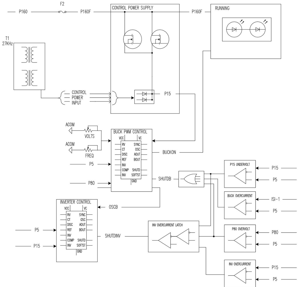
Figure 2. GDPA Board Control and Protection Block Diagram
