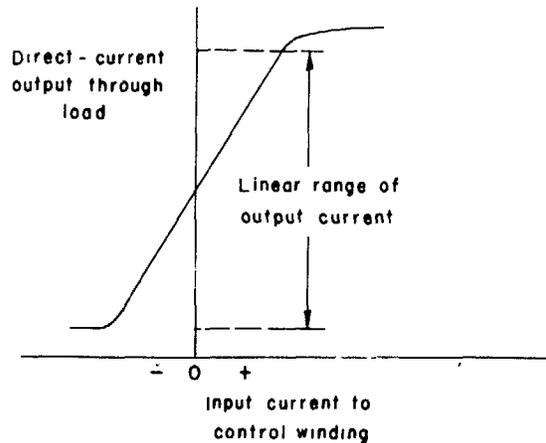
Fig. 8. Characteristic curve of a magnetic amplifier
