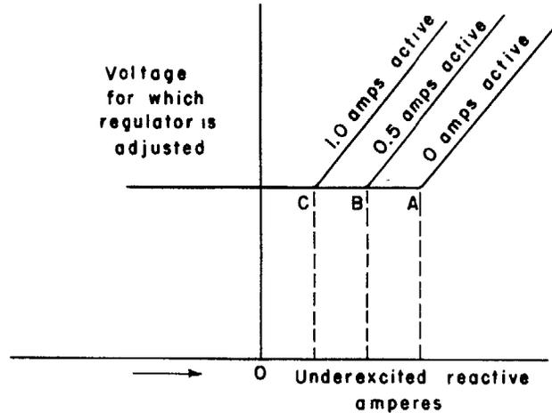
Fig. 13. Curves of underexcited reactive amperes vs. regulator voltage showing how limit-start point is changed as a function of active current
