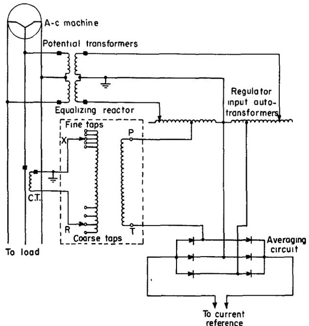
Fig. 14. Equalizing-reactor connections
