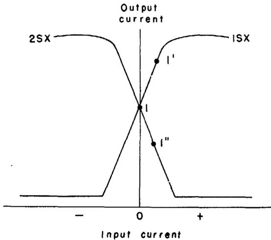
Fig. 10. Characteristic curves of first-stage balanced magnetic amplifier
