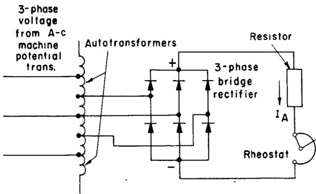
Fig. 1. Elementary diagram of the averaging circuit
