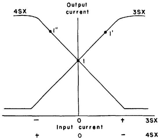
Fig. 11. Characteristic curves of second-stage magnetic amplifier
