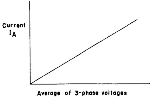
Fig. 2. Curve of averaging-circuit output current vs. average three-phase potential-transformer voltage
