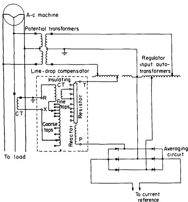
Fig. 15. Line-drop compensator connections
