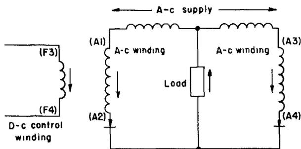
Fig. 7. Elementary diagram showing windings of a magnetic amplifier
