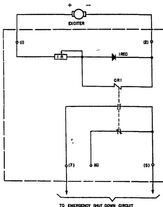
Fig. 17. Exciter voltage relay panel
