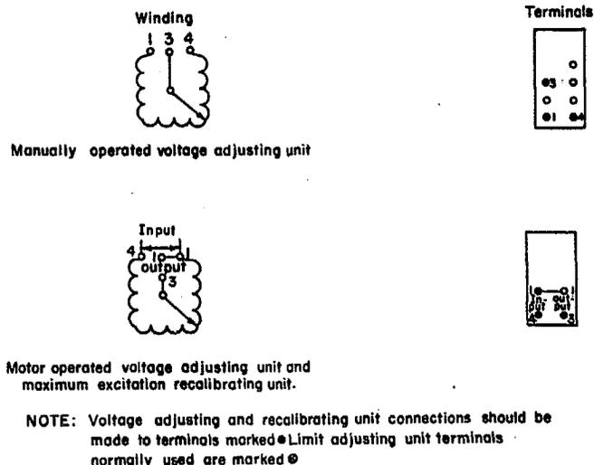
**Fig. 16. Variable transformer internal connections**
