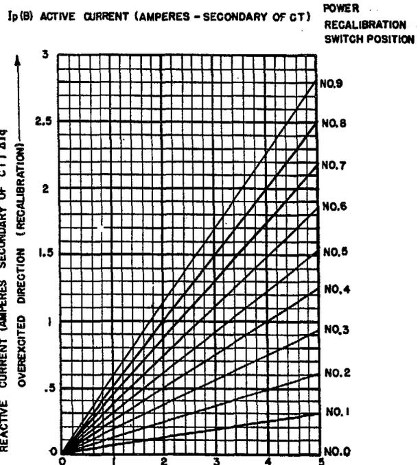
Note: For frequencies other than 60-cycle see appropriate curves supplied with the equipment.
