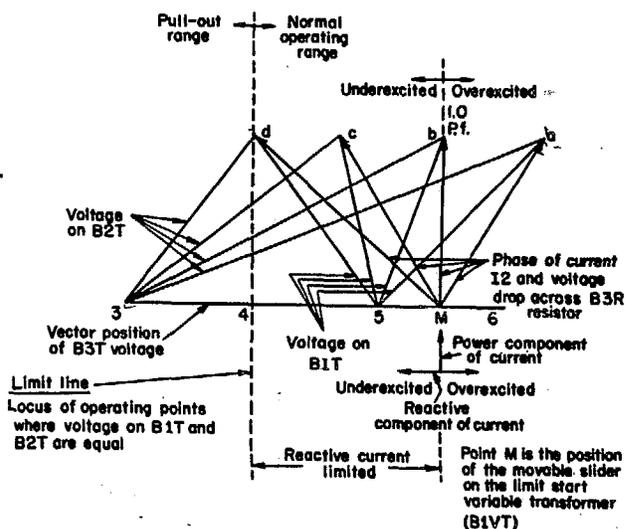
Fig. 6. Vector diagram for reactive-ampere sensitive circuit without power recalibration reactance in circuit
