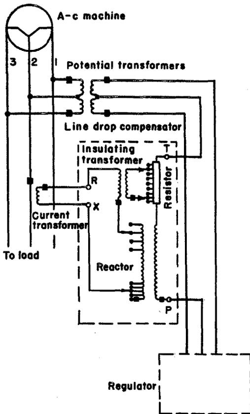
Fig. 14. Line-drop compensator connections
