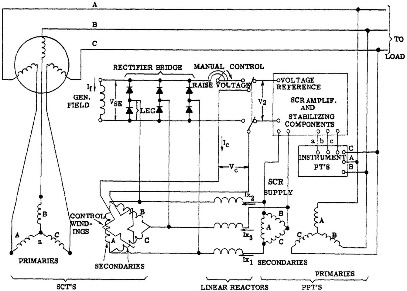
Figure 1. Simplified Static Exciter-Regulator System
