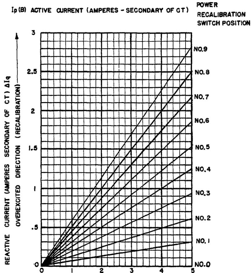
Figure 11. Calibration of Reactive-Ampere Power Recalibration Limit Circuit
