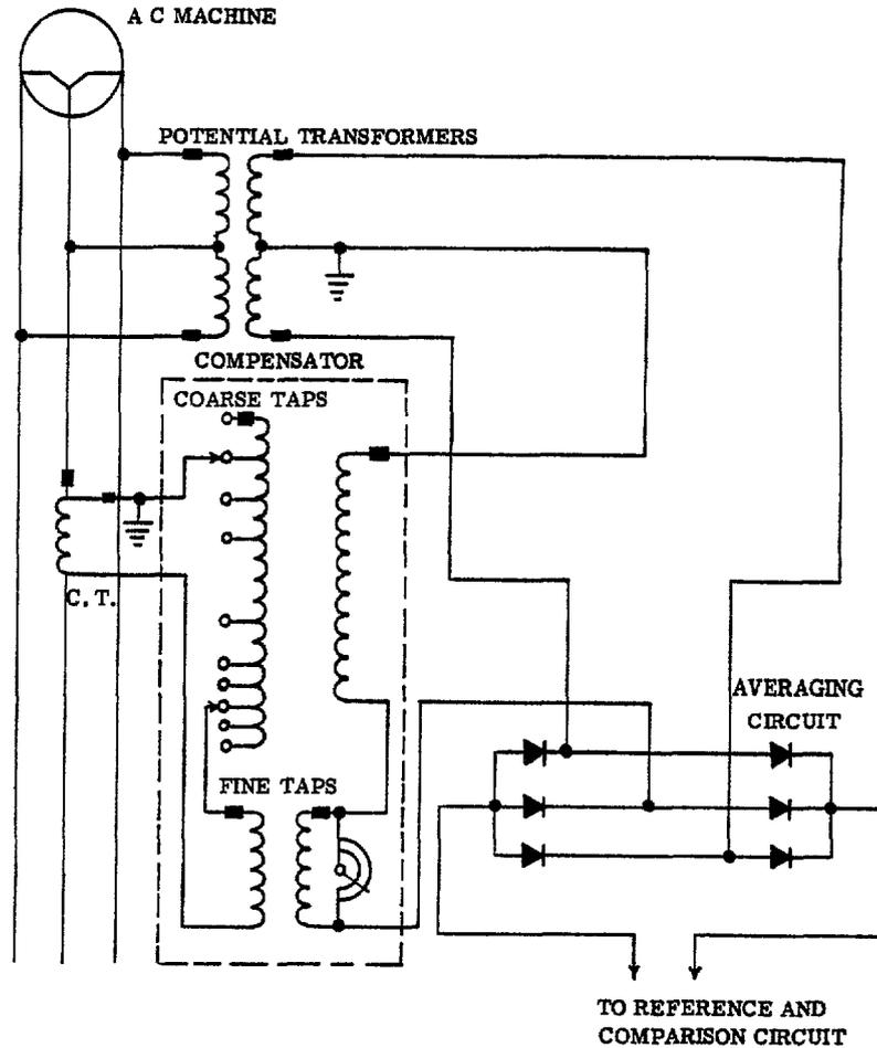
Figure 9. Active-and-Reactive Current Compensator Connections
