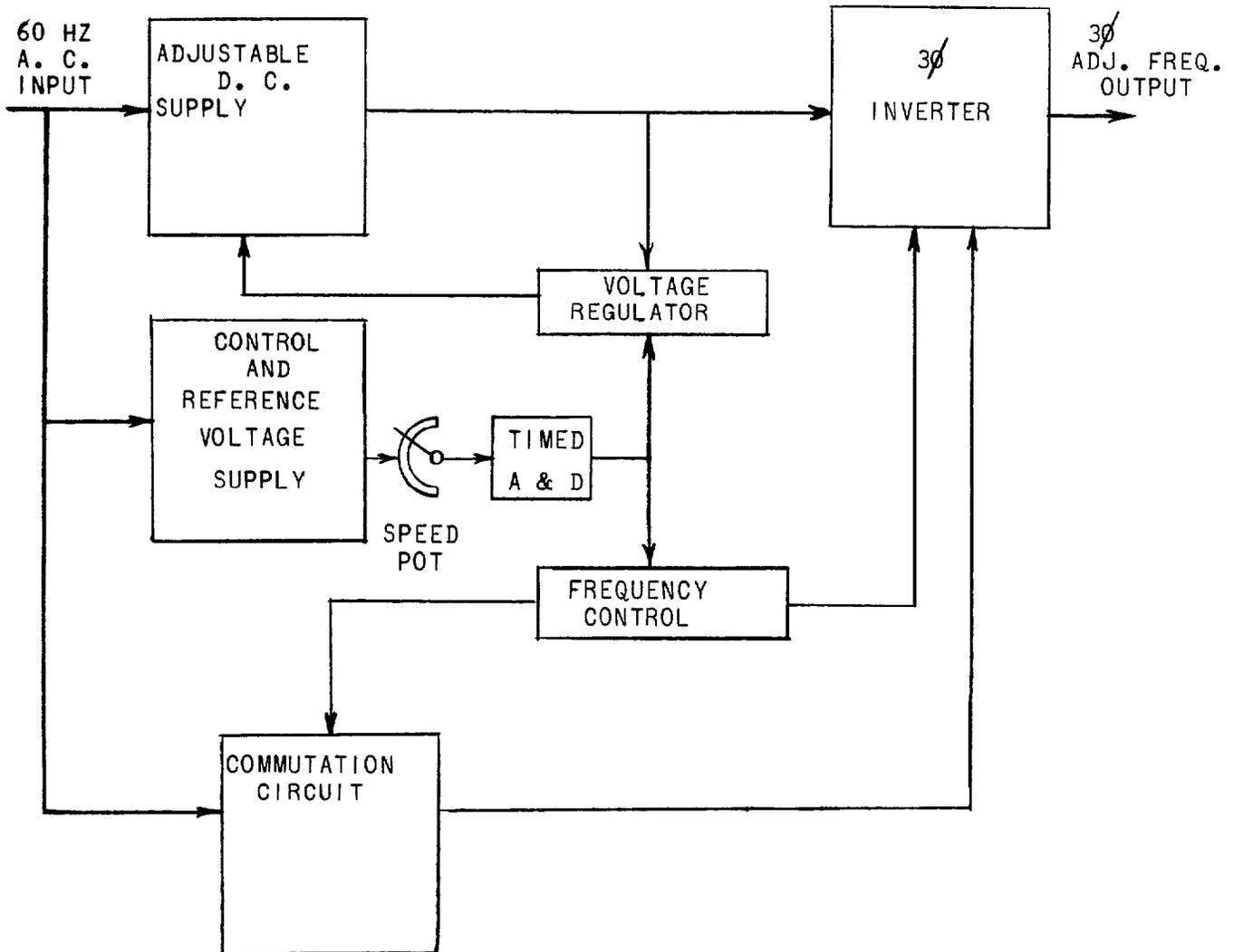
Figure 2. Power Unit Block Diagram
