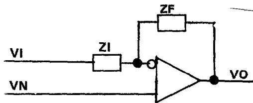
The output of an operational amplifier is short circuit proof and will swing a minimum of  $\pm 10$  volts with a 2K ohm resistive load. Capacitive loads will cause oscillation unless driven by the buffered output of OA3 or OA4 (Tabs 12 and 9X).
