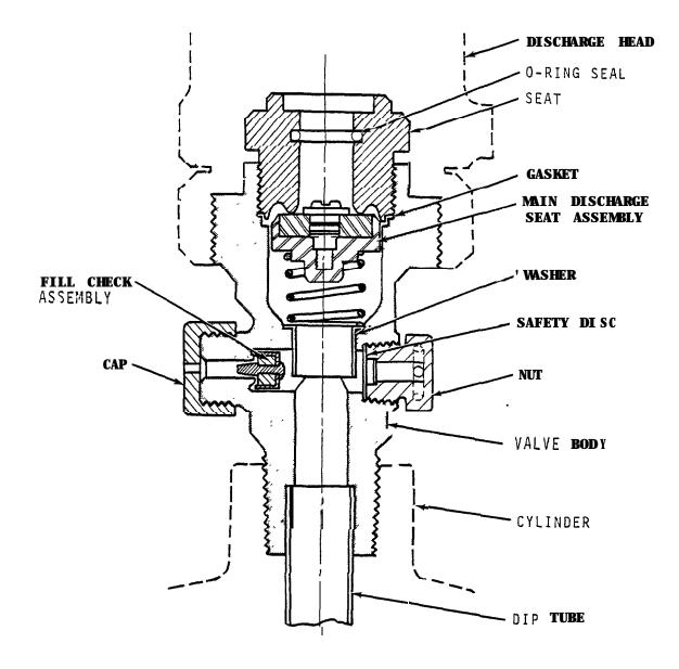
Figure 7. Cylinder Valve and Dip Tube.
