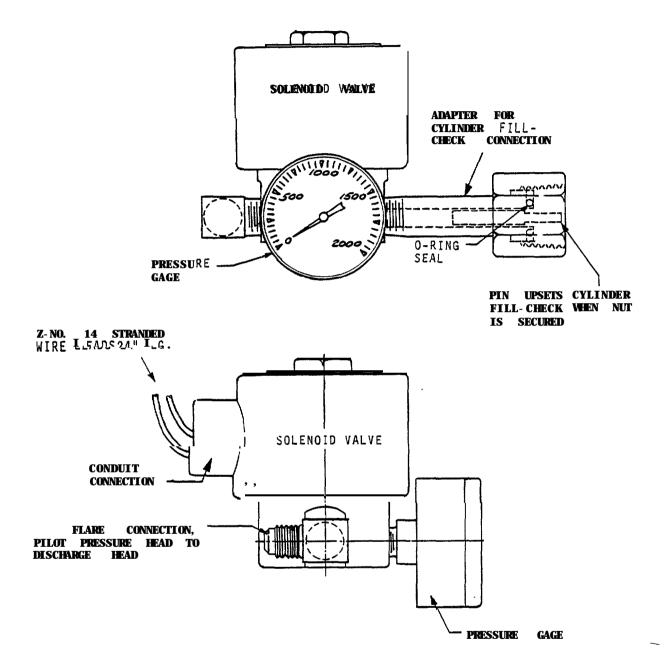
Figure 1. Solenoid Pilot Valves 45CR-1 and 45CR-2.
