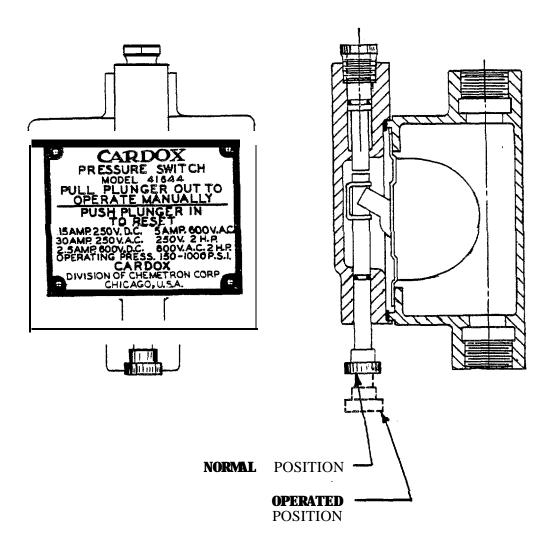
Figure 8. Pressure Switch 45CP.
