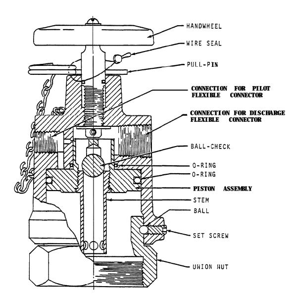
Figure 4. Pilot Operated Heads.
