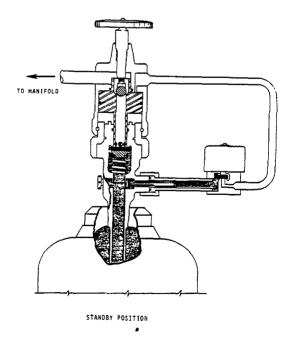
Figure 24. Pilot Cylinder Discharge Heads.
