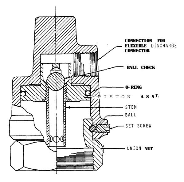
Figure 5. Pneumatic Operated Heads.
