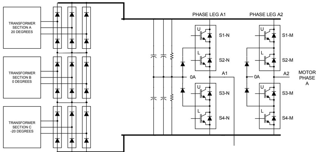
Figure 2. Power Converter Phase Diagram
