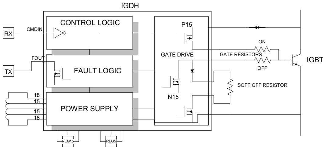
Figure 3. IGDH Subassembly Functional Block Diagram
