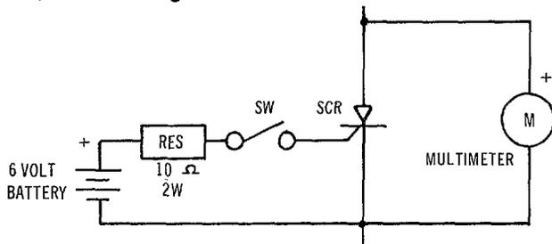
The multimeter is selected to read ohms on the 1K scale, and is connected to read the forward resistance of the SCR. When switch SW is closed, the forward resistance of a good SCR will change from a high value (100K to infinity) to a low value (1 to 10K). When the switch is opened, a good SCR will revert to its high forward resistance or blocking state. A faulty SCR will not switch, remaining in either an open or a conducting state.
