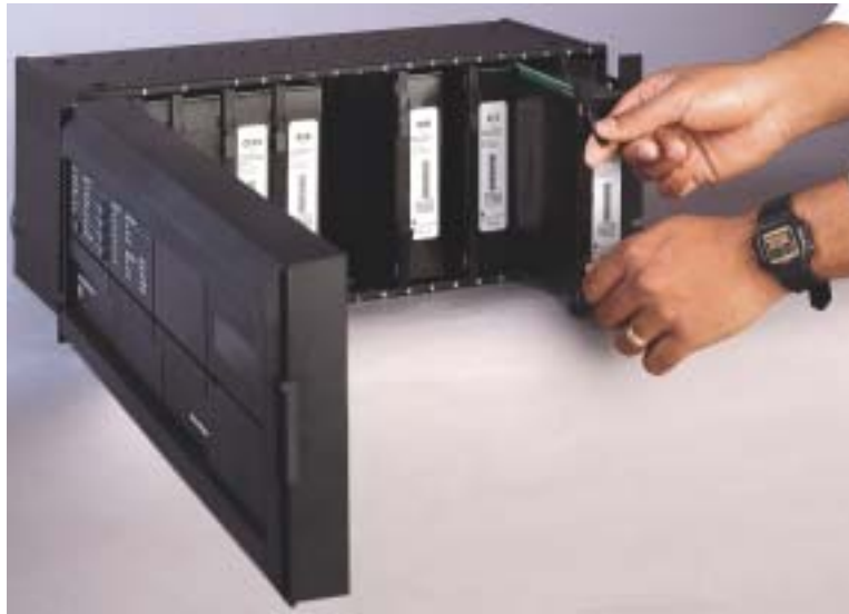
Figure 3-5: UR MODULE WITHDRAWAL/INSERTION
